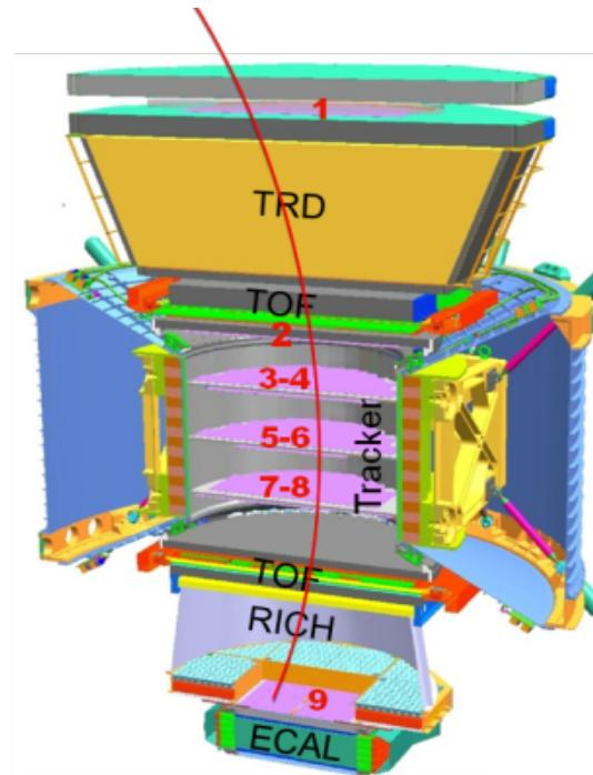
1. TRD (transition radiation) to separate  $e^\pm$  from  $p^\pm$
