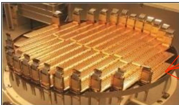
Electromagnetic Calorimeter (ECAL)
