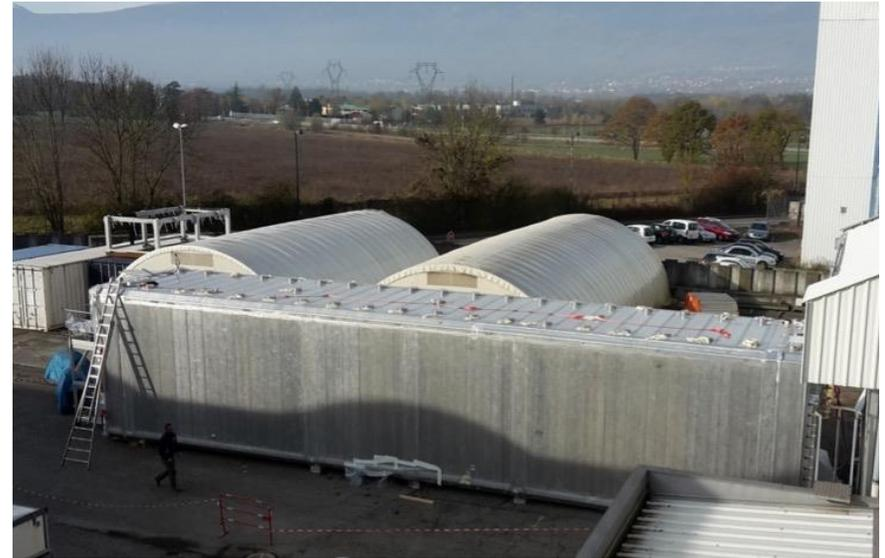
First cold vessel ready to house TPC. Leak tightness verified to  $<10^{-7}$  mbar l/s. Structural test on the vessel by pumping down to 20 mbar. All measurements agree with calculation: 11 mm max. deformation.
