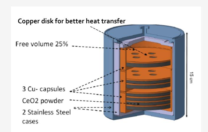
From spent nuclear fuel from Research Reactor purification calcination separation processes CeO<sub>2</sub> powder Pressed up to density of 3 -5 g/cm<sup>3</sup> Put inside the <u>c</u>opper capsule inside the two welded containers Inserted in the byological shield
