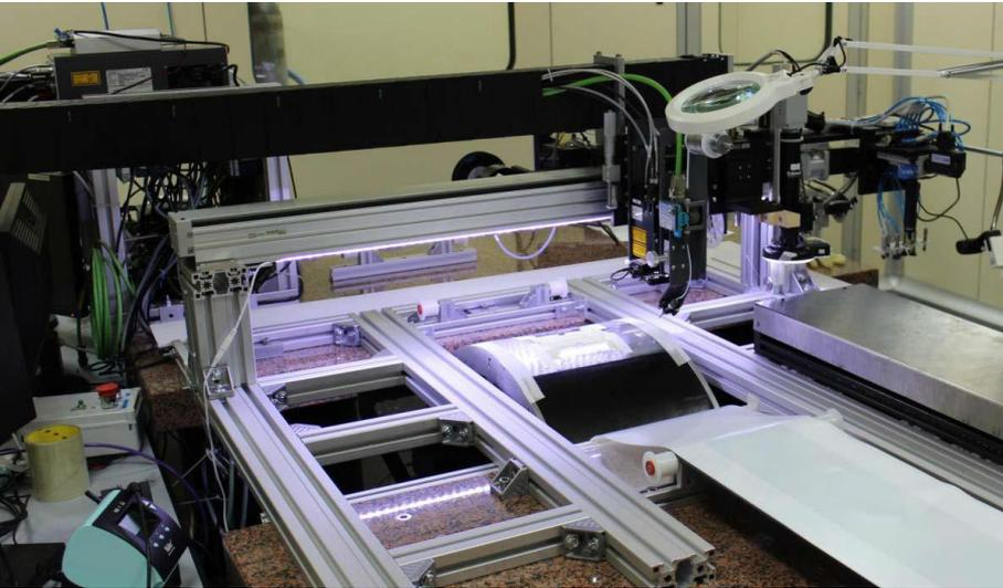
Automated wiring machine in Lecce. Wires mounted on frames and connected to Printed Circuit Boards (PCB) and sent to Pisa for **elongation tests** and **final mounting** on chamber structure.
