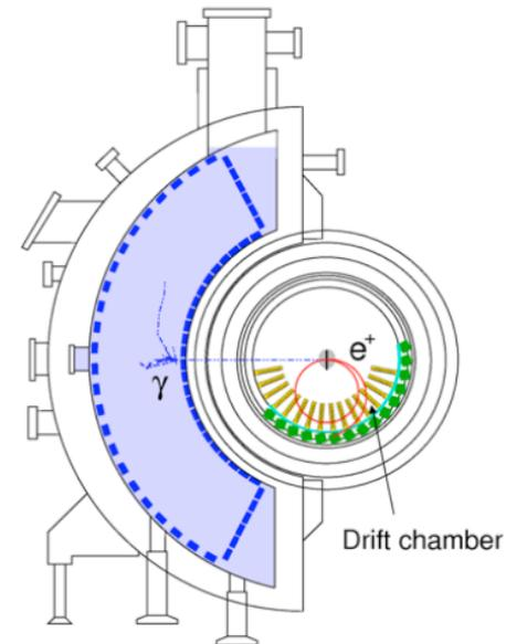
**LXe photon detector:** measurement of photon energy, impact point and timing
