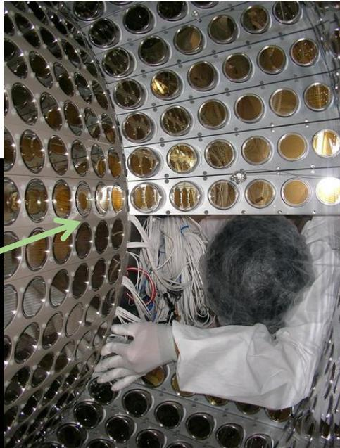
900 l Liquid Xenon photon detector.
