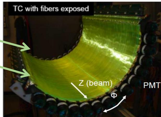
15 x 2 scintillator bars with fine mesh PMTs at both ends.
