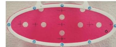
16 DCH with staggered anodic wires and cathodic strips in Vernier pattern. Gas mixture **He:C<sub>2</sub>H<sub>6</sub>=50:50**
