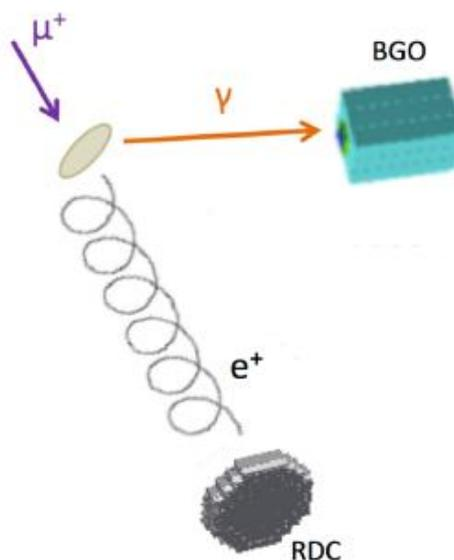
BGO detector used to replace LXe detector
