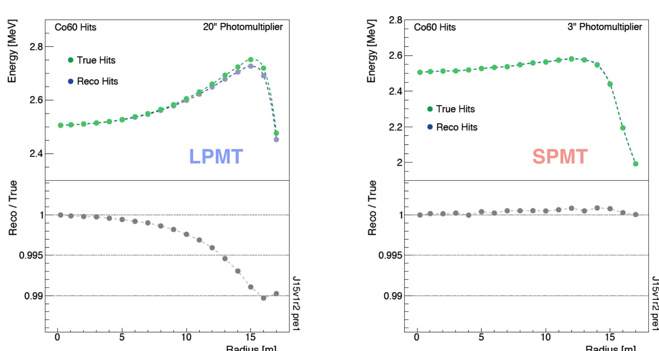
Simulated  $^{60}\text{Co}$  calibration campaign at different radii. The reconstructed energy with LPMT is biased compared to MC, while the bias can be corrected by the SPMT measurement.
