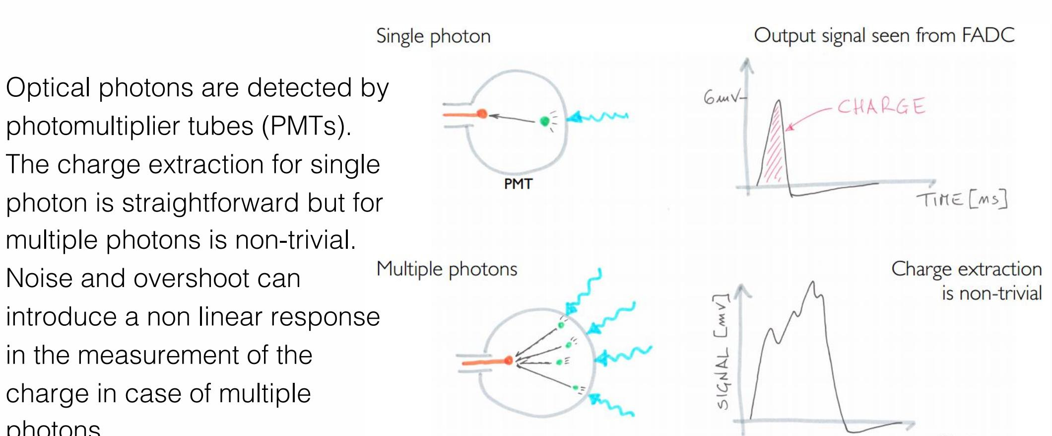
Three ways have been tested to reconstruct the PMT charge based on the sampled waveform with overshoot and noise simulated
