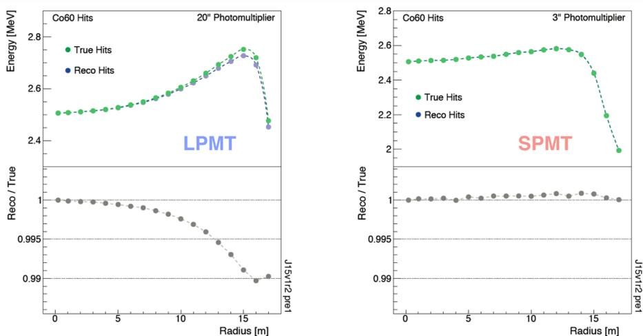
Simulated <sup>60</sup>Co calibration campaign at different radii. The reconstructed energy with LPMT is biased compared to MC, while the bias can be corrected by the SPMT measurement.
