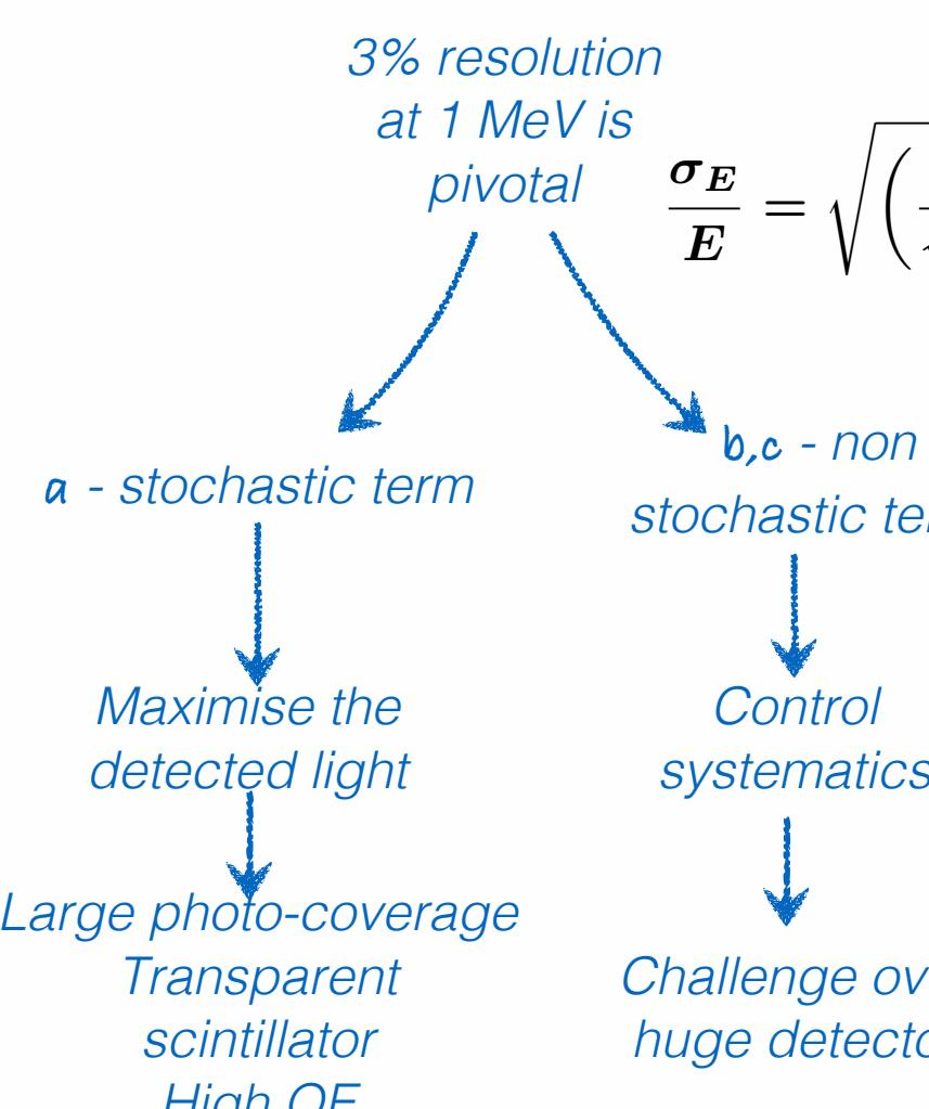
The large Liquid Scintillator (LS) volume and the large (20") PMT's surface imply an unprecedented PMT dynamical range which represents a challenge for the control of the systematic uncertainties.
