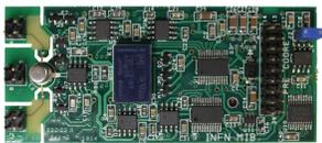
Figure 5: Photograph of the preamplifier
