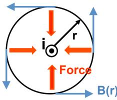
**Red arrow**: focusing force received by the electron beam within an active plasma lens is represented by the red arrow
