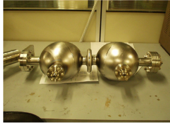
Figure 1: Prototype tuneable detector cavity (variable cell to cell Coupling), Bulk Niobium.
