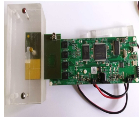
2.5x2.5cm 2 active area prototype with evaluation kit – ready for test
