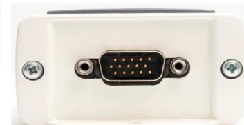
Fig. 4.2: A7501PB Back panel with DB15 connector
