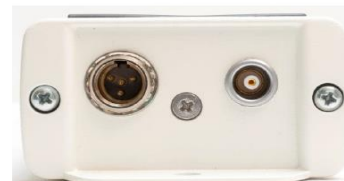
Fig. 4.1: A7501PB Front panel, LEMO HV and 4-pin Mini XLR connectors for Auger IMON and temperature remote inputs
