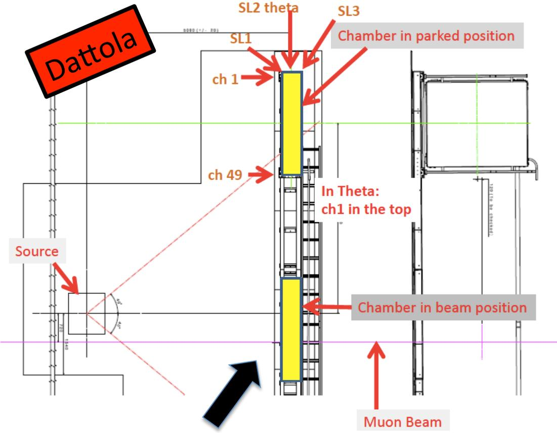
MB1 chamber under test
