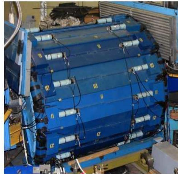
High-resolution NaI calorimeter with excellent tracking and PID
