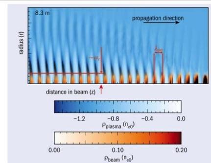
*Fig. 1. Simulation of a self-modulated proton bunch resonantly driving plasma wakefields sustained by the plasma-density perturbation. The plasma density is shown increasing from white to blue and the proton density increasing from yellow to dark red.*
