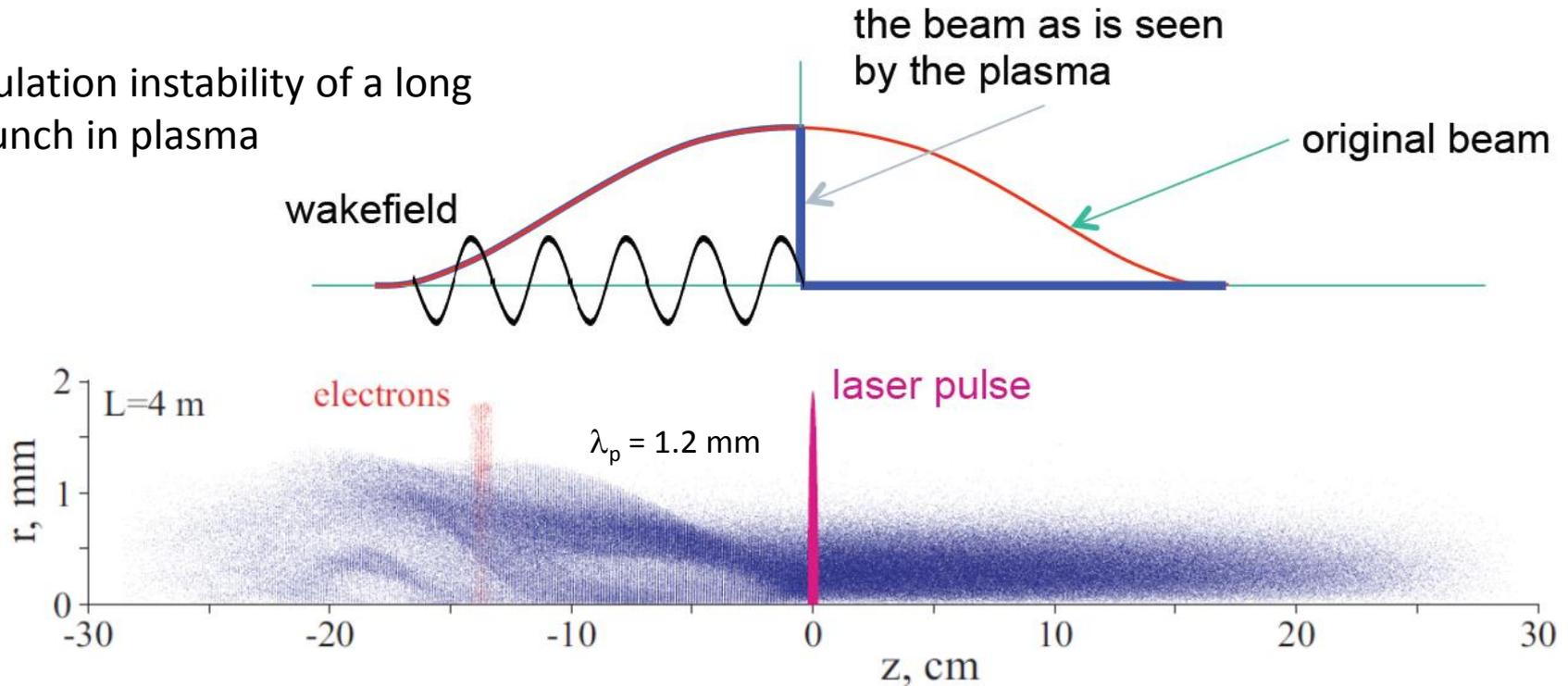
**Self-modulated proton bunch** resonantly driving plasma wakefields.
