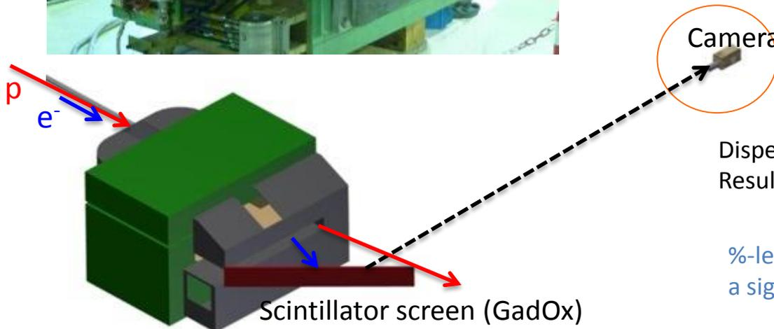
Dispersed electron impact on scintillator screen.
