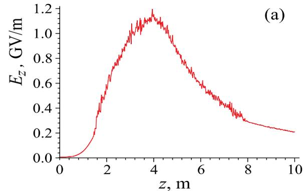
Maximum amplitude of the **accelerating field  $E_z$**  as a function of position along the plasma. Saturation of the SMI at  $\sim 4\text{m}$ .
