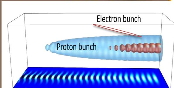
Electron acceleration based on modulated proton driven wakefield acceleration !
