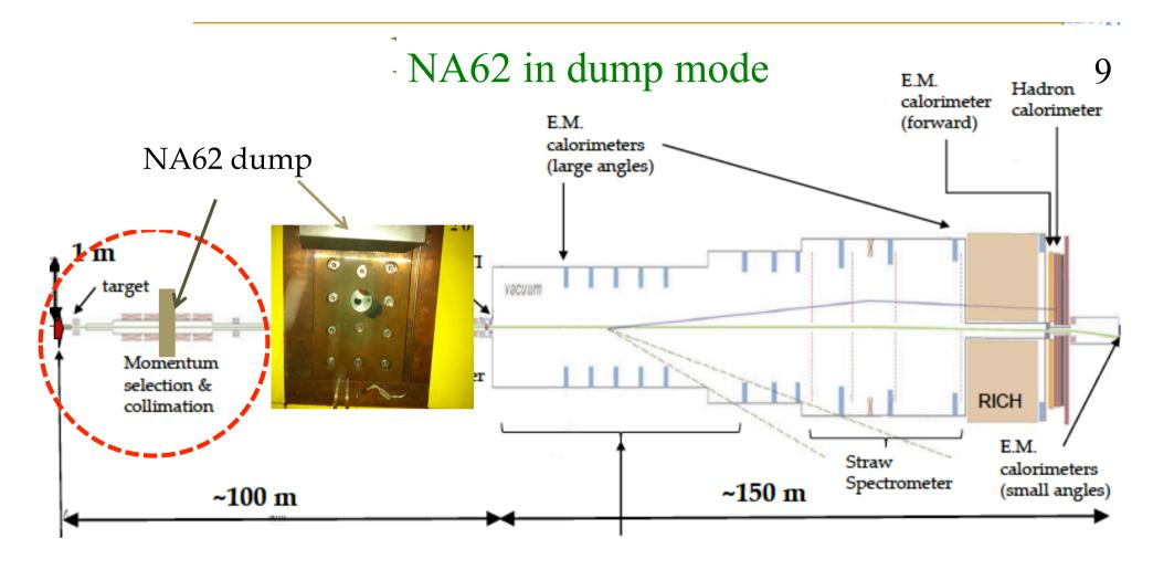
The target is followed 25-m downstream by a 1.6-m long, water-cooled, copper collimators, `Target Attenuator eXperimental areas' (TAXes) offering a choice of bores of different apertures. The TAXes can act as a dump (10.7  $\lambda_{I}$ ) :
