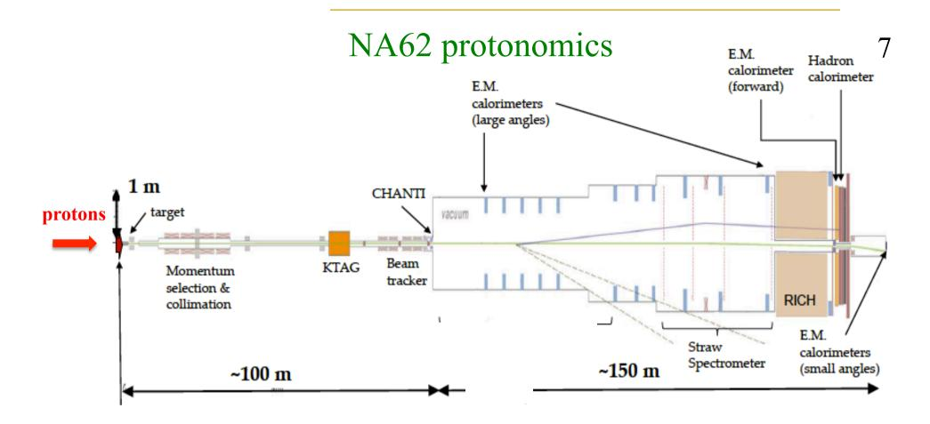
SPS proton 400 GeV 10<sup>12</sup> p/s 3.5 s spill
