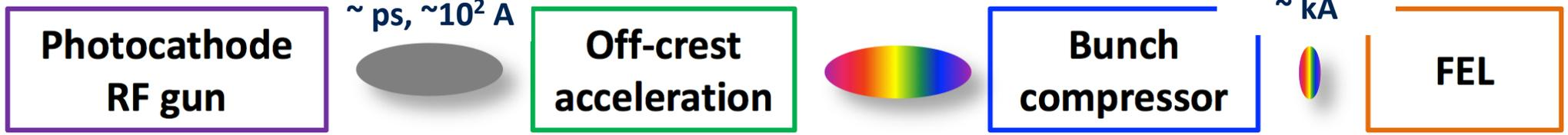
$$\begin{pmatrix} z_1 \\ \delta_1 \end{pmatrix} = \begin{pmatrix} 1 & 0 \\ R_{65} & R_{66} \end{pmatrix} \cdot \begin{pmatrix} z_0 \\ \delta_0 \end{pmatrix} = \begin{pmatrix} 1 & 0 \\ h_1 & \frac{E_{0c}}{E_{1c}} \end{pmatrix} \cdot \begin{pmatrix} z_0 \\ \delta_0 \end{pmatrix}$$
