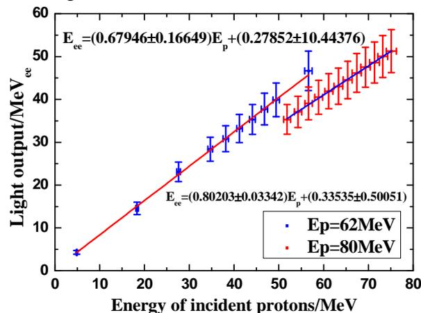
**Fig. 1** Measured light output for YAP:Ce scintillator expressed in MeVee, as a function of the incoming proton energy
