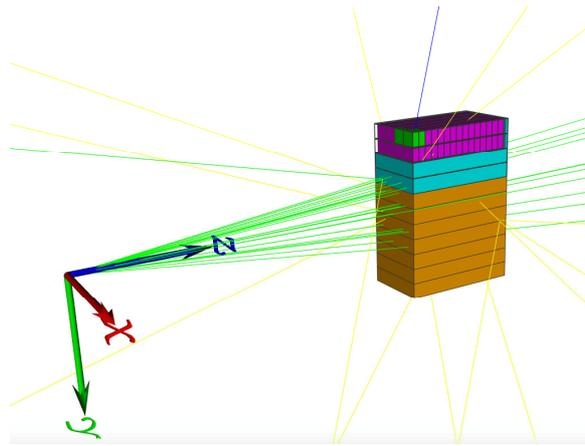
Fig. 1 GEANT4 simulation for neutron irradiation of a Multi-Grid Detector.
