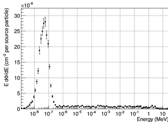
**Fig. 1** Neutron energy spectrum inside the photo-converter cavity calculated by MCNP6 simulation. The thermal peak represents the 80% of the total flux, while the fast neutron component (above 0.2 keV) is below the 5%.
