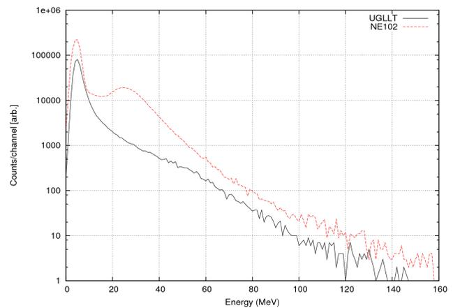
Figure 2: The calibrated energy spectra from the UGLLT (black) liquid scintillator and NE102 (red) plastic scintillator.
