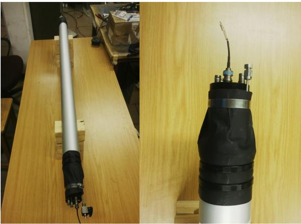
Figure 1: A photographic picture of the liquid scintillation detector setup.
