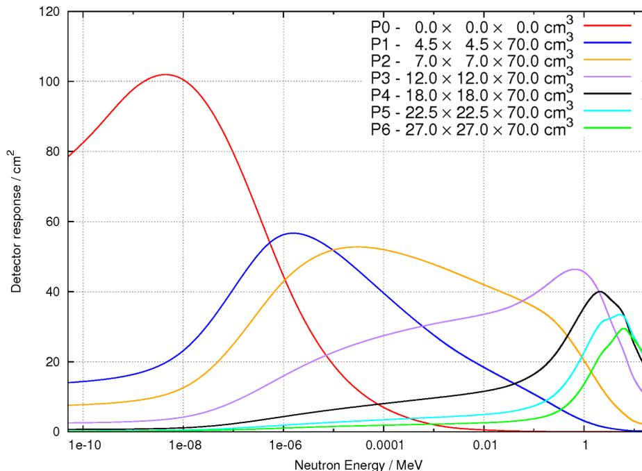
**Fig. 1** Detector responses for the seven polyethylene shielded  $^3\text{He}$  counter tubes calculated with FLUKA.
