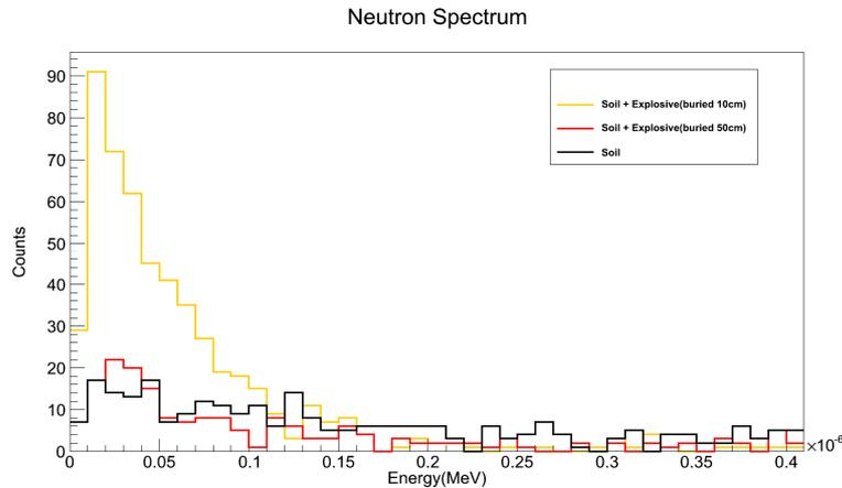
**Fig. 1** Comparison of thermal neutron spectrum of a buried 1000 kg explosive for various burying depths in soil.
