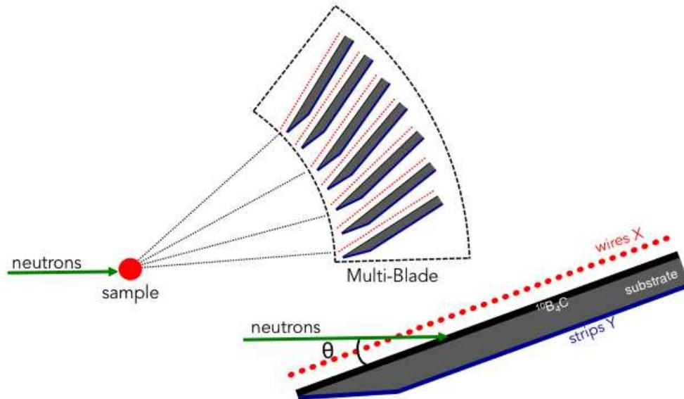
Fig. 1 Schematic view of the cross-section of the Multi-Blade detector made up of identical units (cassettes) arranged one after the other. Each cassette holds a  $^{10}\text{B}_4\text{C}$ -layer and the readout is performed through a plane of wires and a plane of strips.
