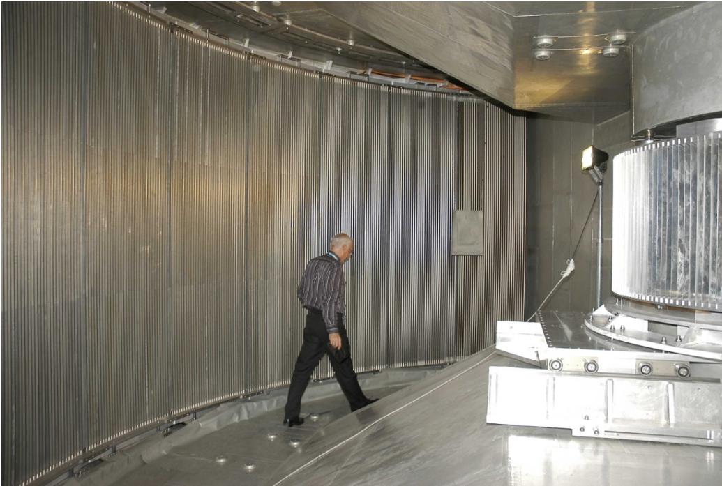
The 30 m 2 detector of the IN5 TOF Energy spectrometer at the ILL
