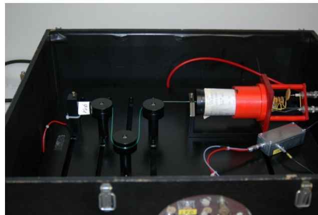
Picture of the test setup for bending the fibers around different diameters in total 360°
