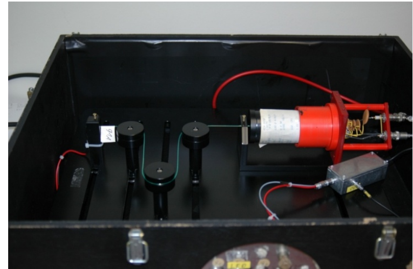
Picture of the test setup for bending the fibers around different diameters in total 360°
