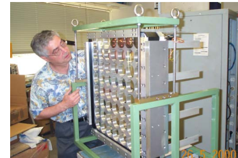
Assembling of the PMTs
