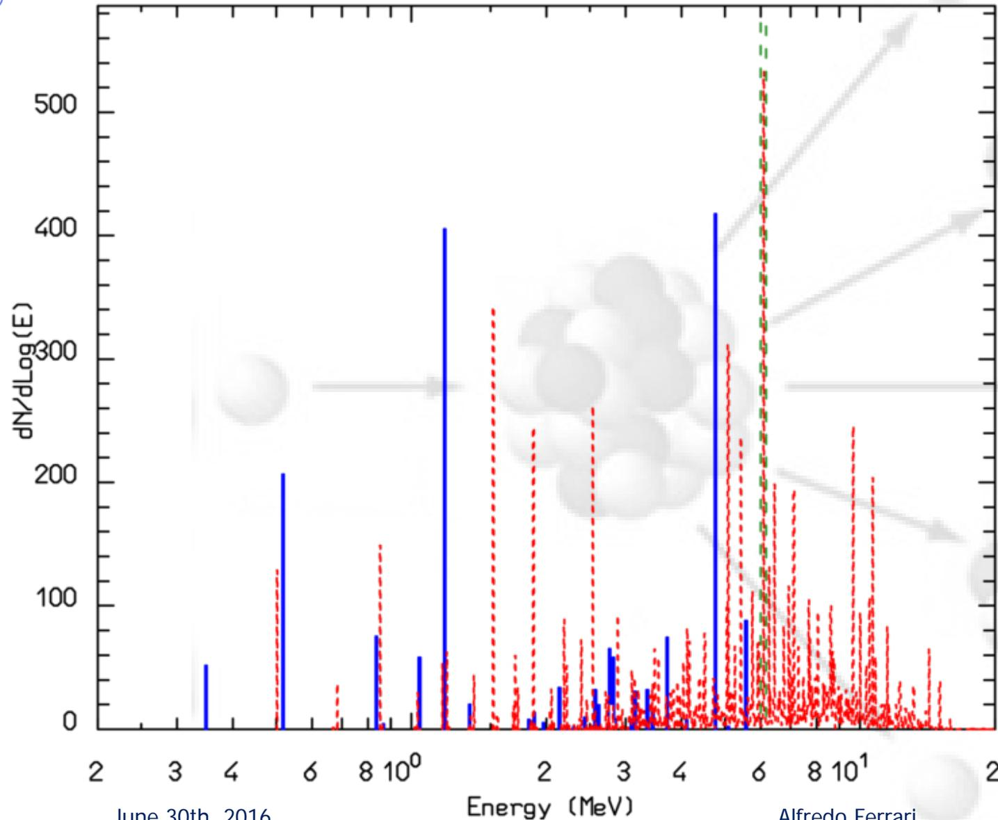
Liquid Argon experiments are popular for neutrino physics. Icarus @ LNGS was supposed to measure also solar  $\nu$ 's and the main background was neutron capture by  $^{40}\text{Ar}$
