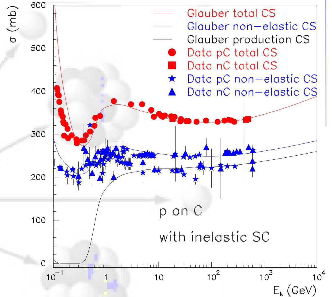
Proton (Neutron) Carbon cross sections computed in self-consistent Glauber approach accounting for inelastic screening
