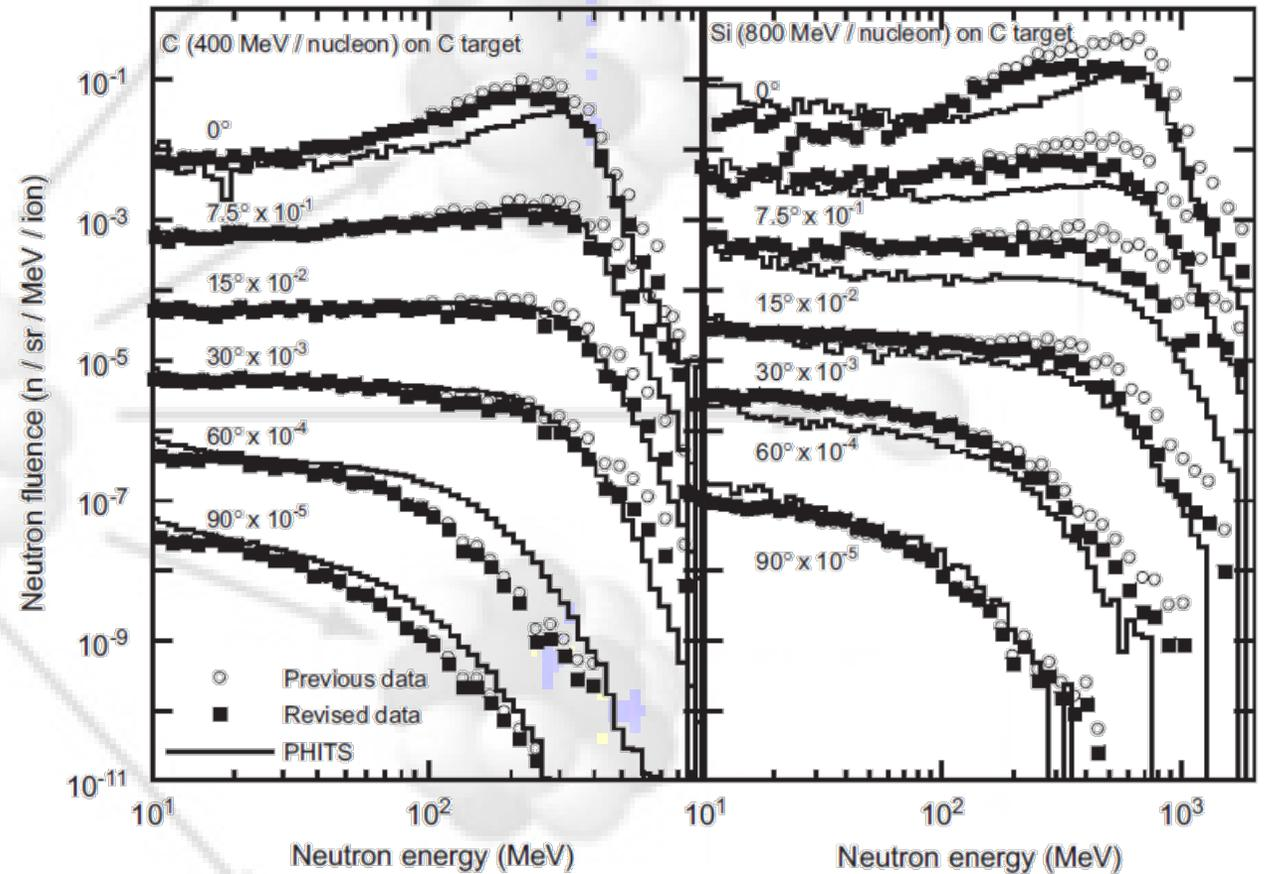
Fig. 5. Revised neutron spectra for 400-MeV/nucleon C-ion and 800-MeV/nucleon Si-ion bombardment of C targets.
