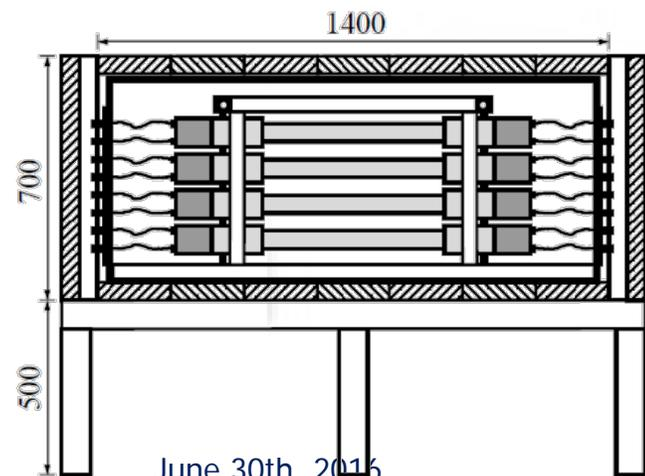
The neutron *background* at LNGS is *very weak* ( $\sim 0.5 \cdot 10^{-6} \text{ cm}^{-2}\text{s}^{-1}$ ,  $E > 1\text{MeV}$ ), while the  $\gamma$  one is "normal"  $\rightarrow$  a very large discrimination required. Achieved by using 32, 1 liter, liquid scintillator (BC501A) detectors, each one wrapped in Cadmium, and using both PSD and delayed coincidence of the fast neutron proton recoils with capture  $\gamma$ 's  $\rightarrow$  then unfolding
