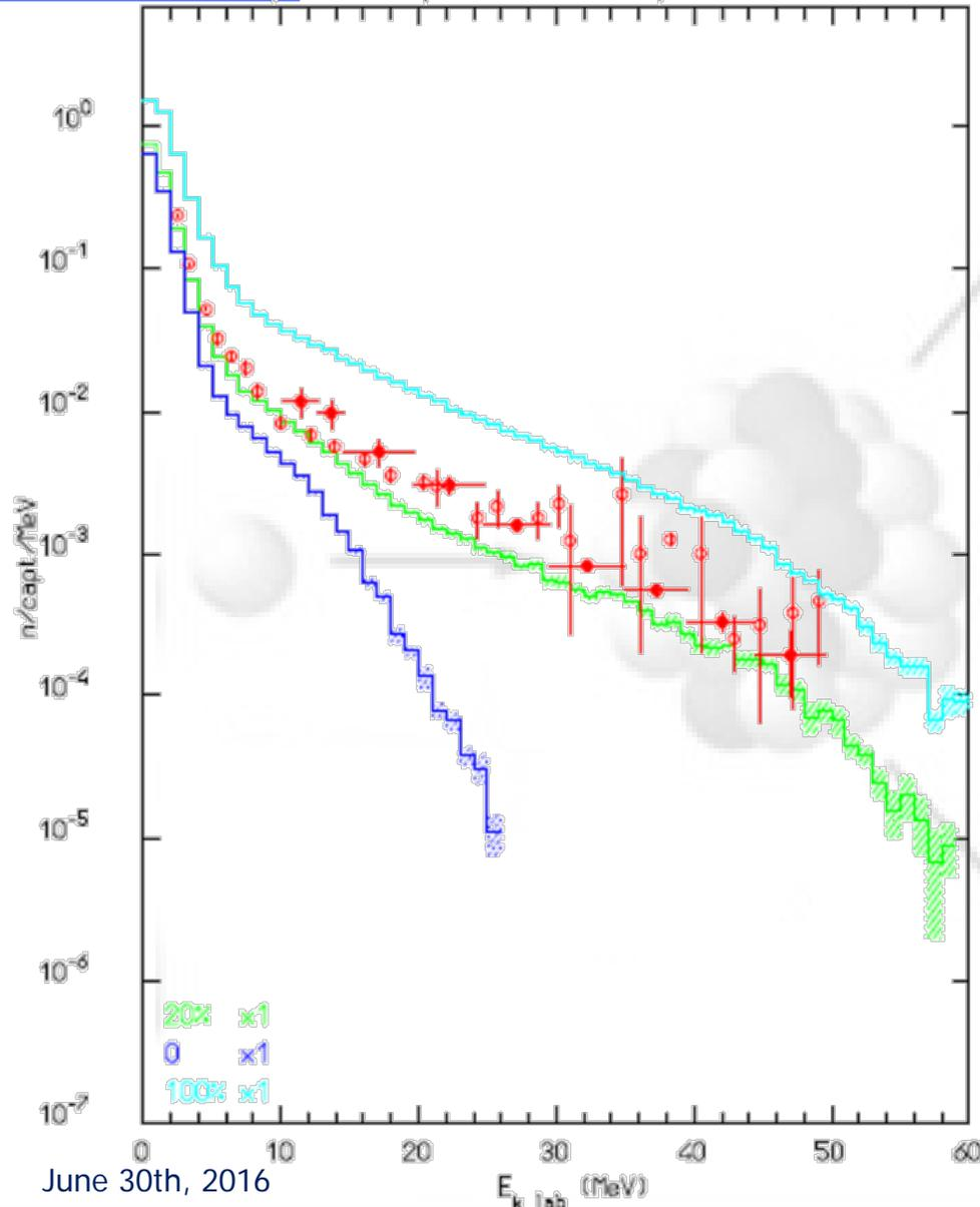
Neutron spectra following muon capture on Lead
