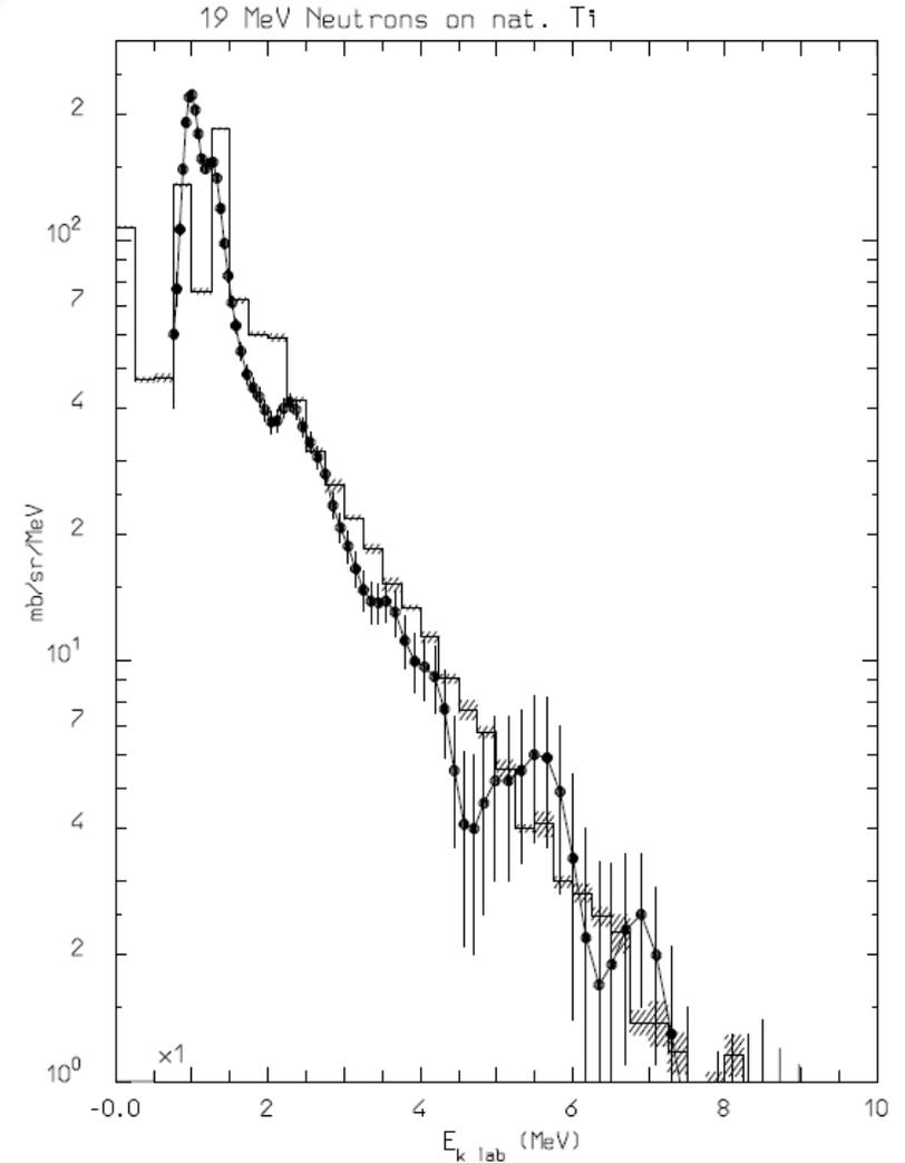
**Fig. 1.** Photon spectrum resulting from the reaction  $\text{Ti}(n,x)$  at 19 MeV. The dashed histogram represents PEANUT results with errors. Dots are experimental data from [34]
