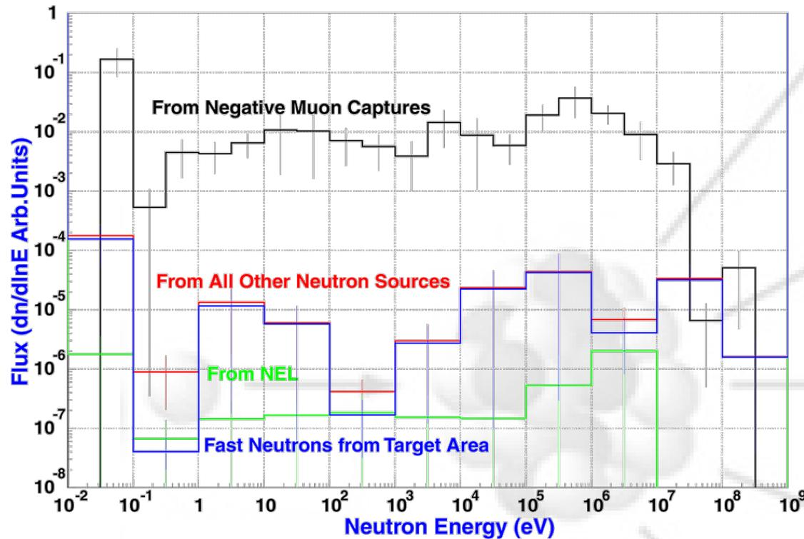
Neutron Fluence in the experimental area divided into the various sources
