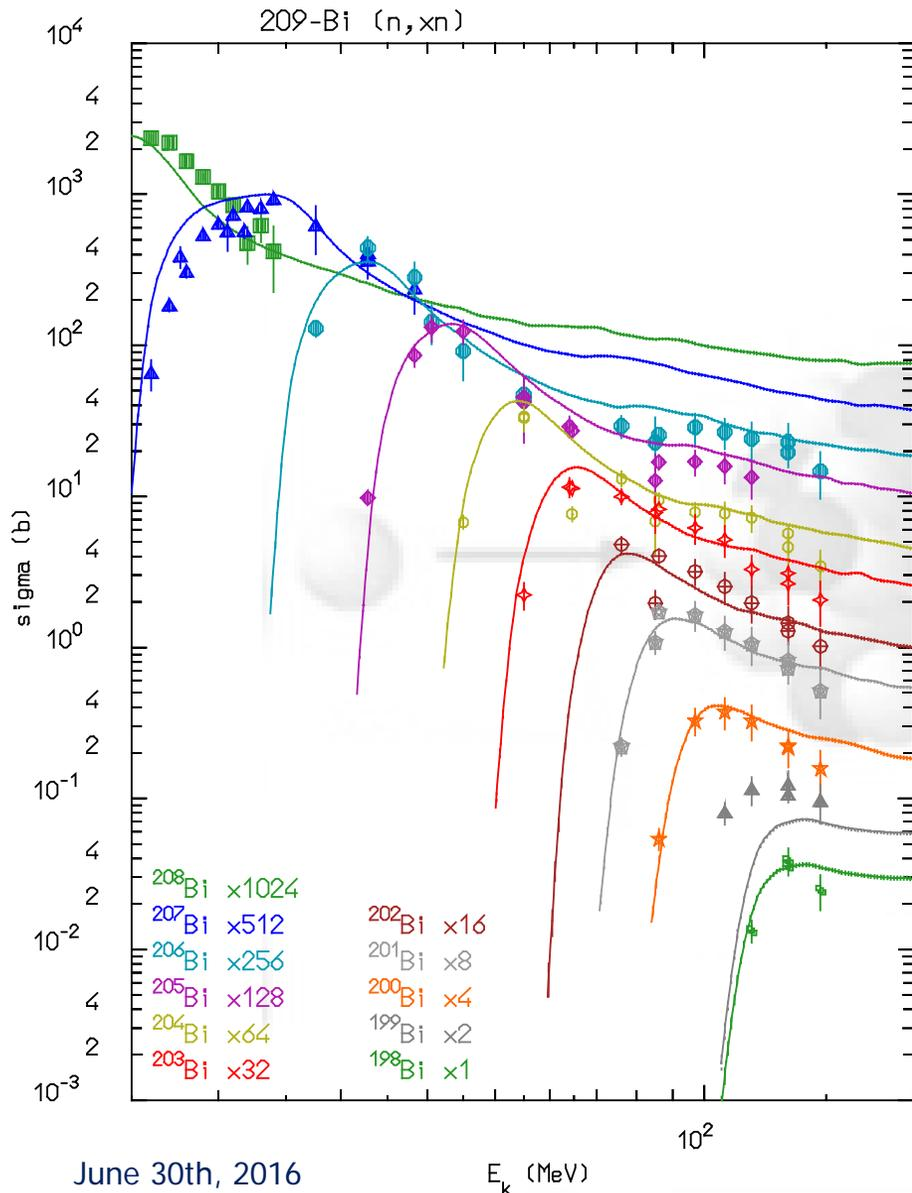
Examples of computed isotope production versus exp.data: FLUKA (lines with dashing) vs exp. data (symbols).
