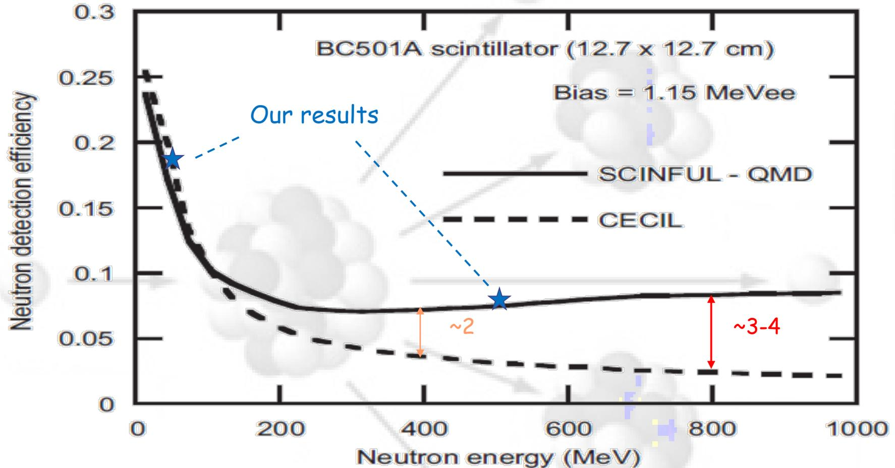
Fig. 1. Neutron-detection efficiency of a BC501A-type liquid organic scintillator with bias of 1.15 MeVee. Solid and dashed lines indicate the calculation results of SCINFUL-QMD and CECIL, respectively. The escaping proton events were eliminated in both calculations.
