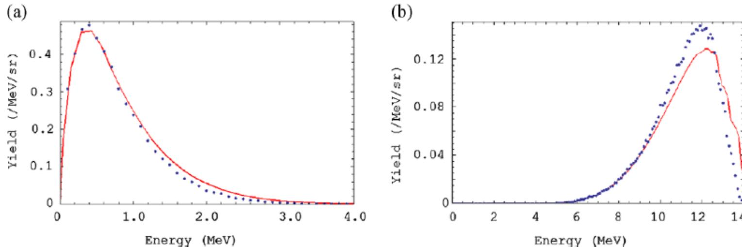
**Fig. 31.** Secondary particle energy spectra of  $^{197}\text{Au}(n,np)$  reactions by 20 MeV neutrons integrated over the whole solid angle. The line represents the original cross-section of JENDL 4.0. (a) Neutron and (b) proton.
