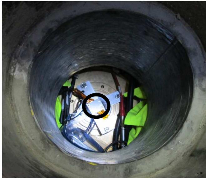
SDD setup in the MPR after-burner
