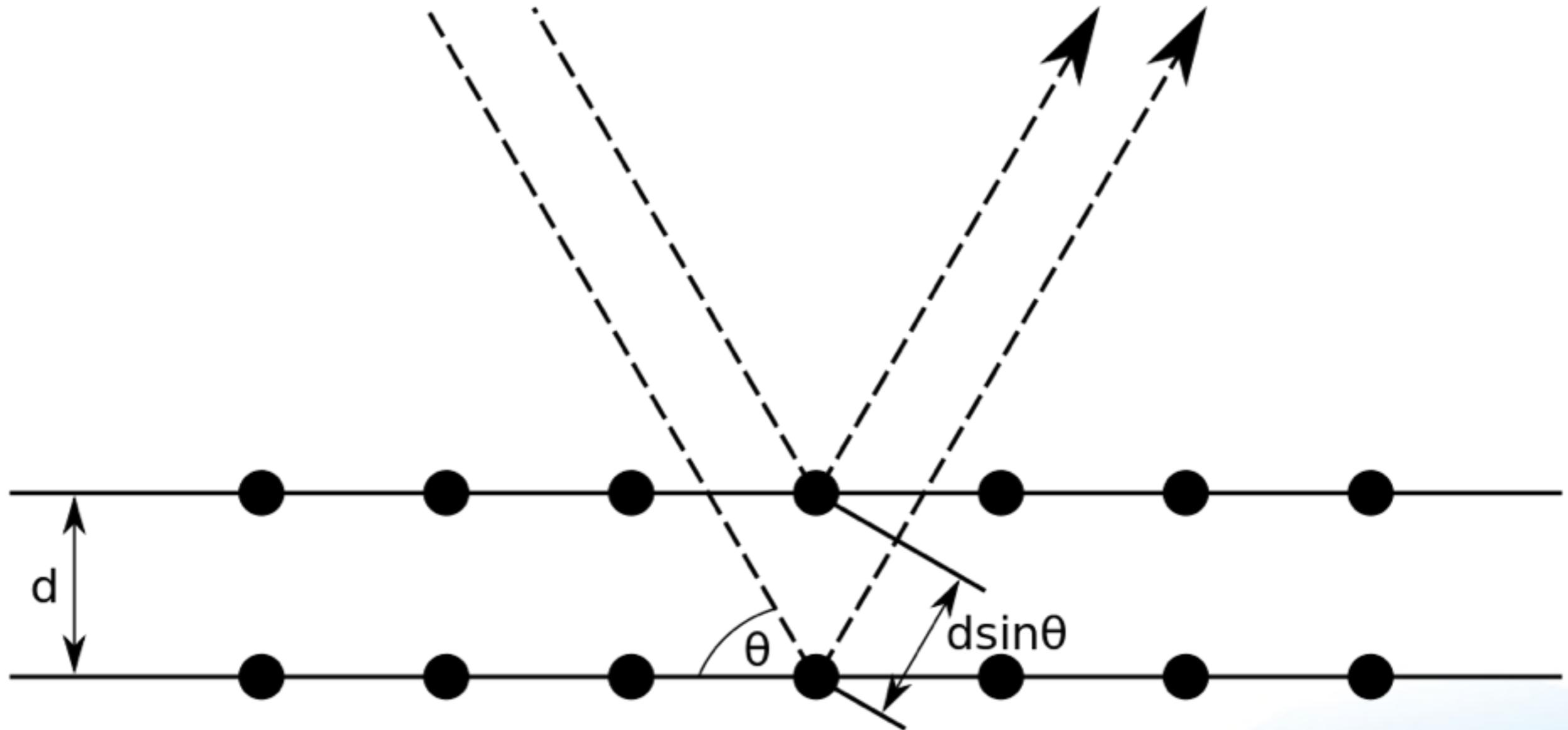
Position and intensity of diffraction peaks gives atomic positions
