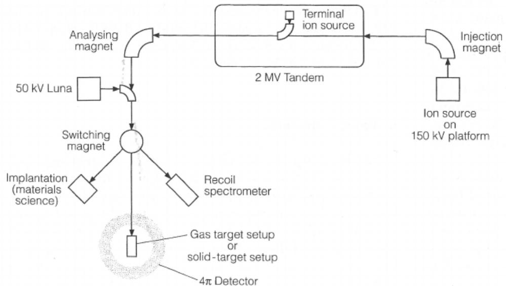
**Fig. 5.** Schematic diagram of the layout of an underground accelerator facility
