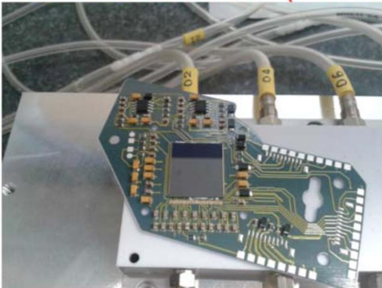
Ultrathin (53 micron) pixel detector for the AeglS beam imaging
