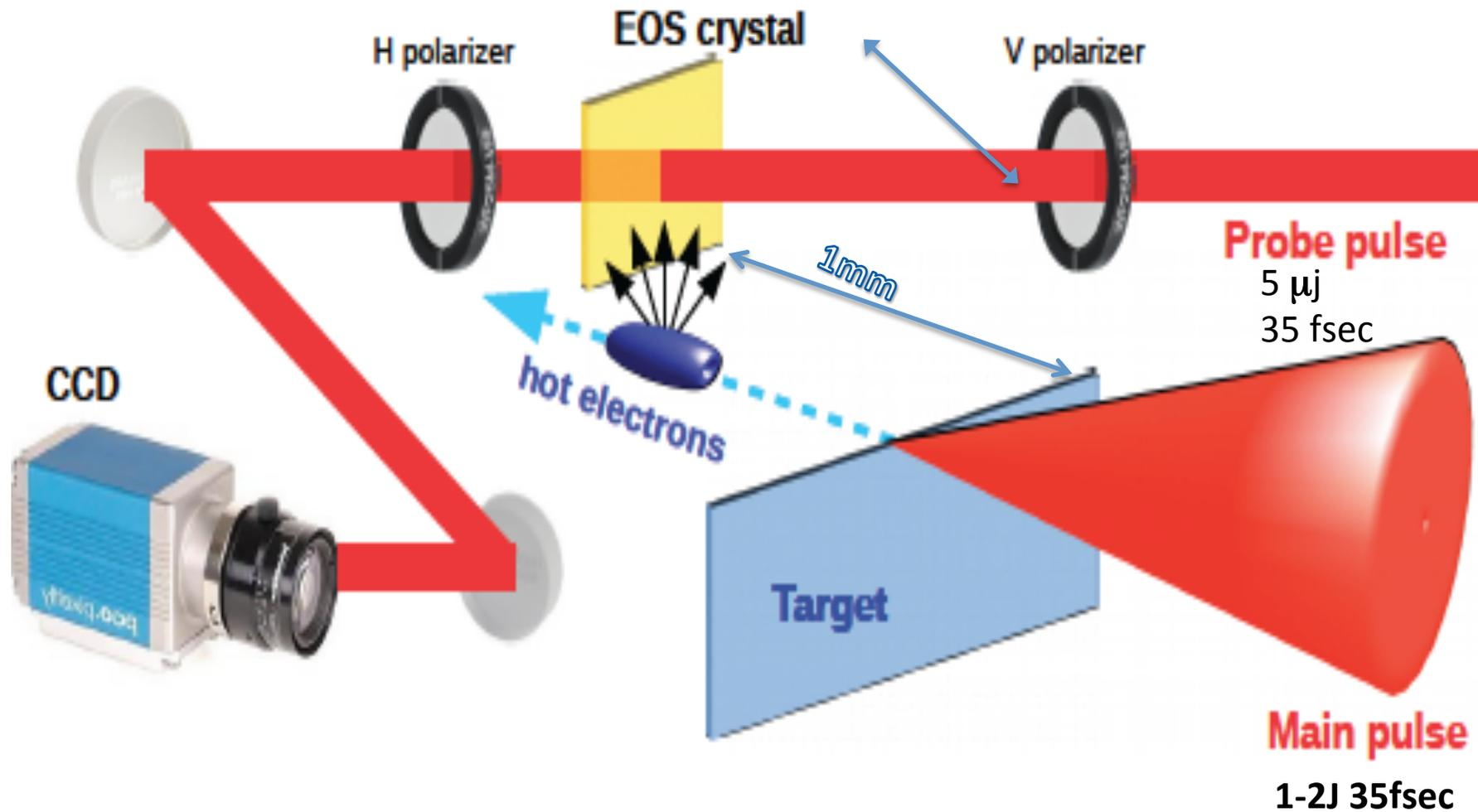
Schematics for measuring quantity and temporal evolution of the escaping electrons
