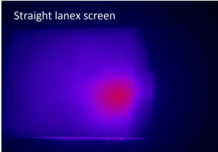
Electrons have been accelerated up to an energy of about 170 MeV in 4 mm Helium gas-jet.
