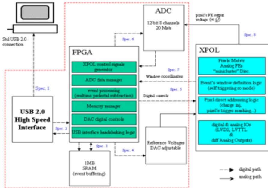
An FPGA is the core of the whole EGSE 0.0
