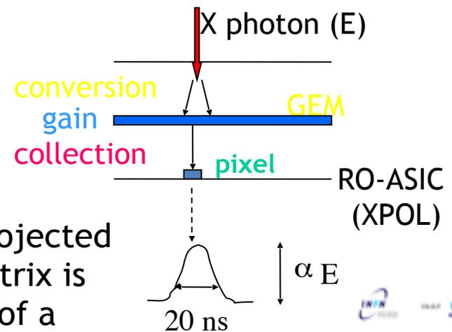
The charge ( $e^-$ ) generated in the avalanche is projected onto the 50 $\mu$ m pitch active pixel matrix. The matrix is indeed formed with the upper-most metal layer of a 0.18 $\mu$ m CMOS ASIC
