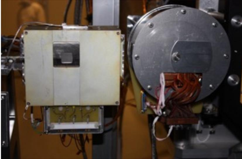
EGSE 0.0 successfully accompanied the GPD through all the Environmental test performed so far: Thermal cycles, Thermo-Vacuum (  $10^{-6}$  mbar), Heavy-Ions survival test...
