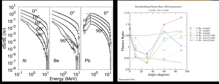
Geant4.10.3.b01: G4EmStandardPhysicsGS (with Goudsmit-Saunderson scattering model for electrons), global production cut for secondary particles of 0.01 mm, dRoverRange 0.05 mm, dFinalRange 0.05 mm.
