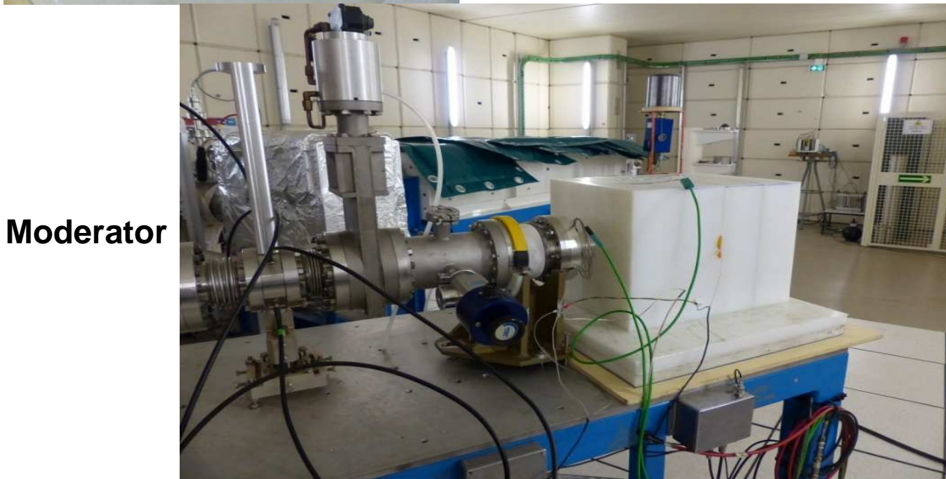
Detector was shielded by polyethylene and B4C
