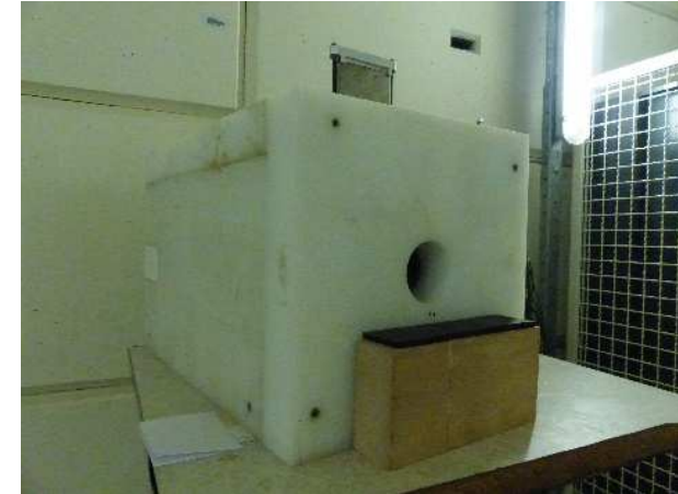
Detector was shielded by polyethylene and B4C
