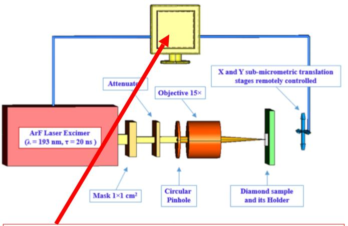
**<u>LabVIEW</u>** software used to remotely control at the same time the laser and the X and Y translation stages operations.
