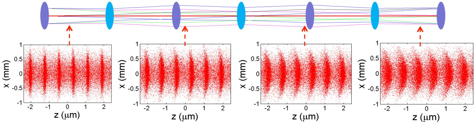
**Particles with larger betatron amplitudes have longer path lengths**
