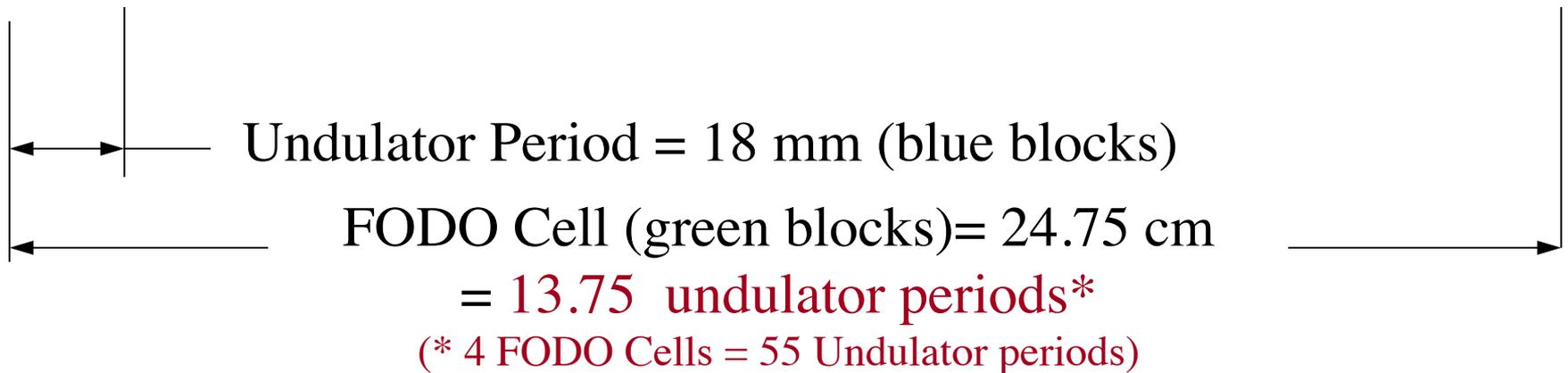
Total Length = 110 Periods = 8 FODO cells, built in two 99 cm long sections + terminations
