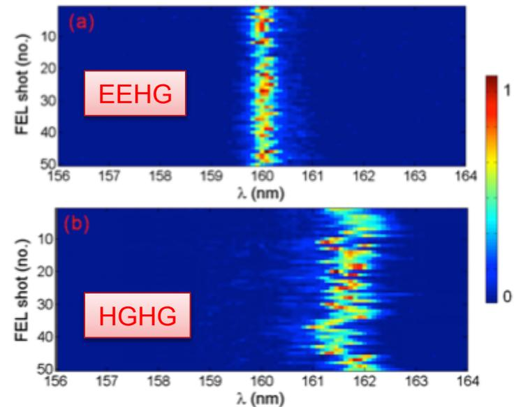
FIG. 7. Fifty consecutive radiation spectra for EEHG (a) and HGHG (b) with a chirped beam. Note, the central wavelength of HGHG signal is shifted by the linear chirp and the bandwidth of the HGHG signal is increased by the nonlinear chirp, while those for EEHG are essentially unaffected.
