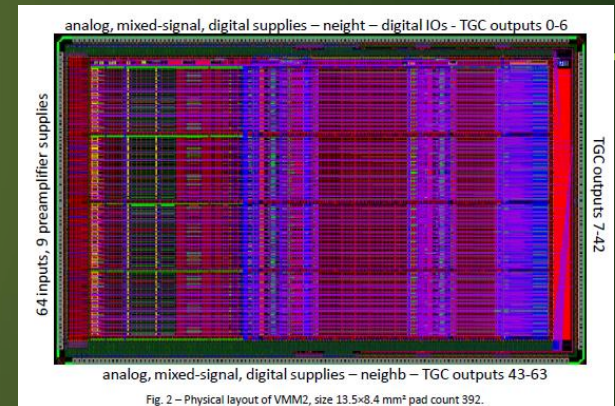
130nm 1.2V 8-metal CMOS technology from IBM
