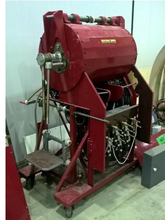
Fig. 1. Magnetic + semiconductor detector conversion-electron spectrometer based on an "old" Siegbahn–Släts magnet used as the electron transporter: (1) beam, (2) target, (3) target-changing system, (4) collimator and current measurement, (5) Faraday cup, (6) lead shield, (7) antiproton baffle, (8) detector, (9) feedthrough, (10) coldfingers, (11) coldtrap, (12) to pump, (13) cylindrical plastic scintillator, (14) light guide, (15) bellows reflector, (16) PM tube.
