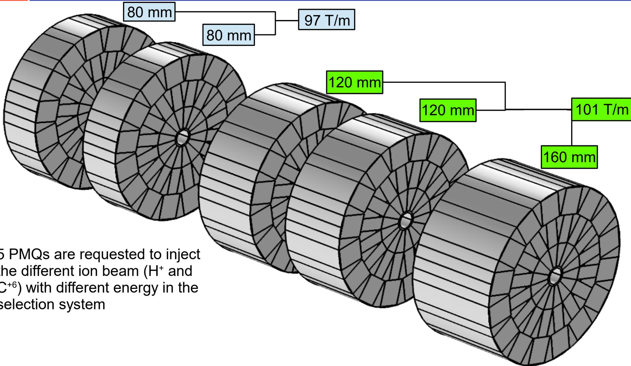
5 PMQs are requested to inject the different ion beam ( $H^+$  and  $C^{+6}$ ) with different energy in the selection system
