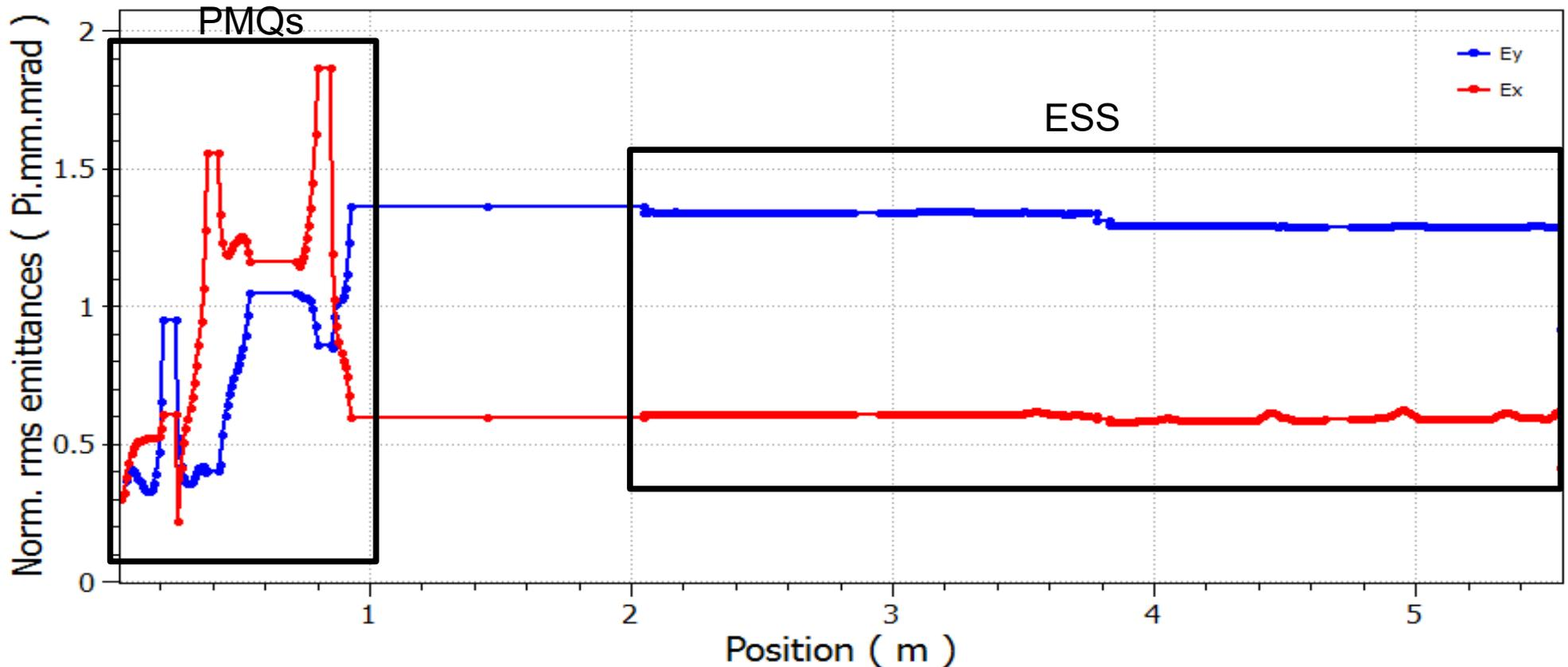
Emittance growth limited to the PMQs system and due to filamentations in the PMQs
