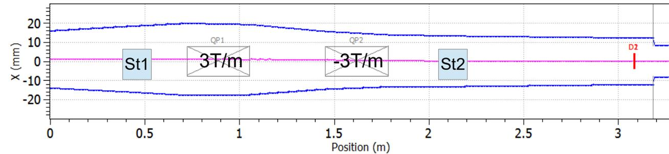
Out of PMQs+ESS used in input for preliminary simulation of last beam-line section
