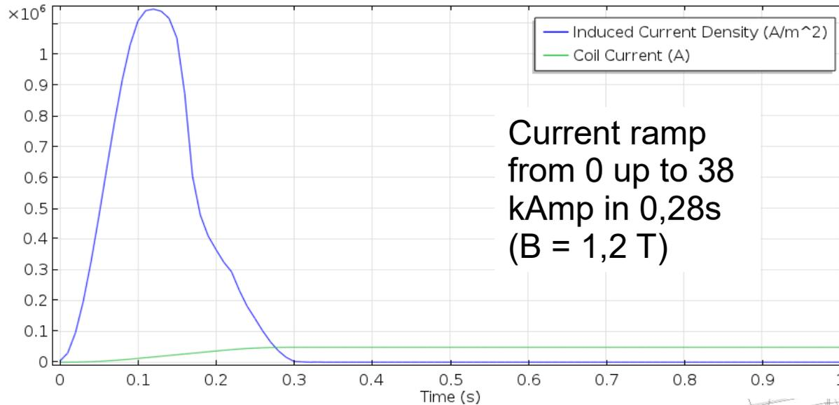
If the current is changed each second (each laser shot) the system could be used as an active energy modulator system - Induced sextupole due to the eddy current on the vacuum chamber can be neglected after 0,31s
