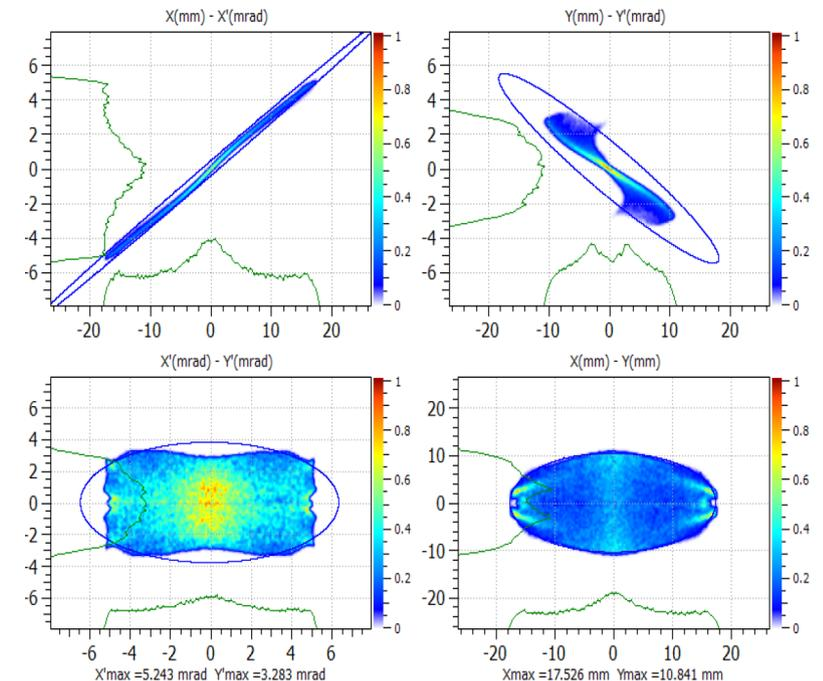
Beam envelope for reference beam 60 MeV protons
