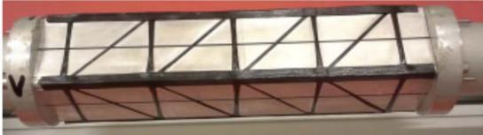
4. Placement of corner L-sections (UD prepreg)
