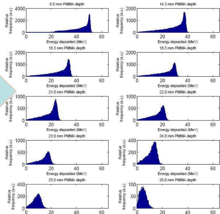
Geant4 proton depth kinetic energy simulation
