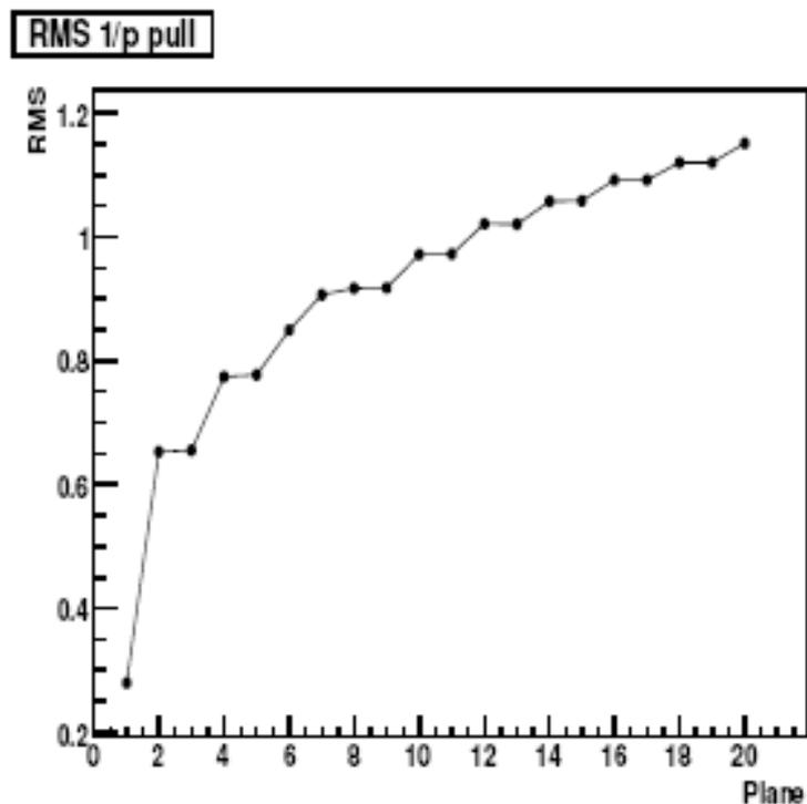
Figure 4: Values of the standard deviations of the  $1/p$  pull variable with truncation parameter  $\delta = 0.9999$  from eq. (15), as a function of the number of the traversed layers. The data refer to 1 GeV pions traversing layers formed by a 1 mm thick Al (Landau distribution) and a 1 cm thick Ar gas (Urban distribution) absorbers at NTP.
