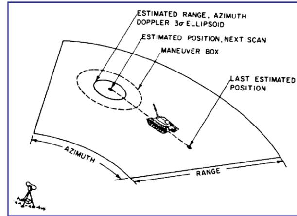
In a radar application, where one is interested in following a target, information about the location, speed, and acceleration of the target is measured at different moments in time with corruption by noise.
