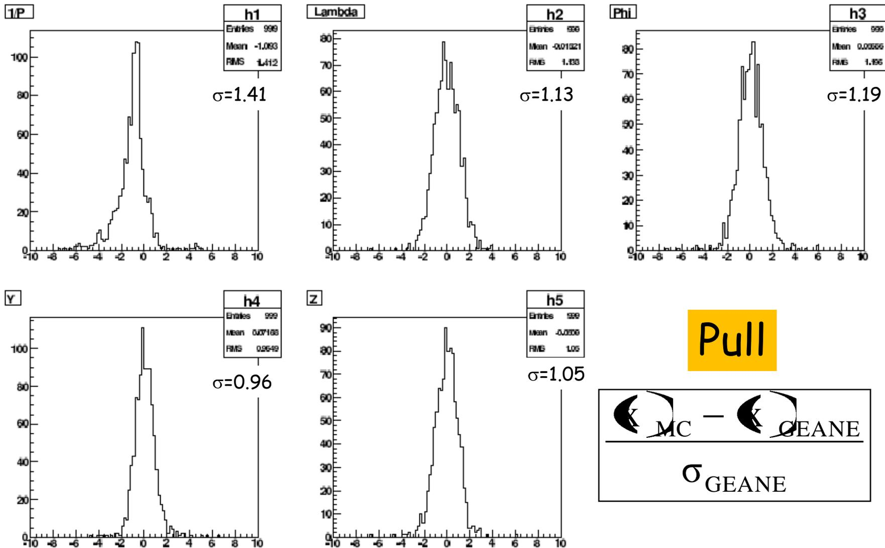
Figure 11: Pull distributions of the 5 track parameters in the case of 2 GeV muons that have passed through the whole detector, just before the PANDA
