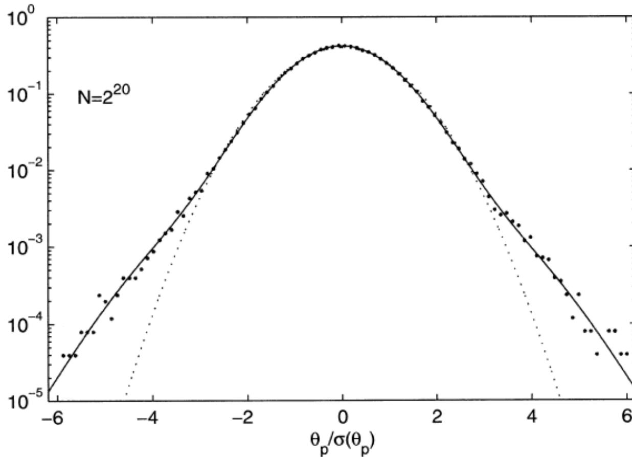
Fig. 3. The density of the projected multiple scattering angle in carbon, in standard measure, for  $N = 2^{10}$  (top) and  $N = 2^{20}$  (bottom). The dots are the frequencies of a simulated sample obtained by summing over single scatters. The dotted line is the density of a standard Gaussian.
