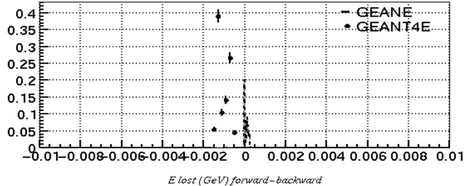
Difference in energy when a 20 GeV track is propagated forwards and then backwards
