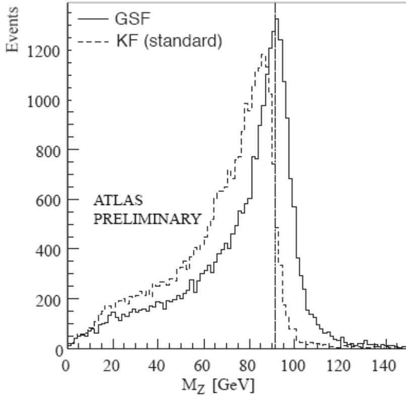
**Figure 6.** Improvement of the  $Z$  mass distribution for  $Z \rightarrow e^+e^-$ , when the electron tracks are (re-)fitted with the Gaussian sum filter instead of the standard ATLAS Kalman filter. In the standard Kalman filter, energy loss is applied only as mean ionisation loss and even approximated as being Gaussian distributed.
