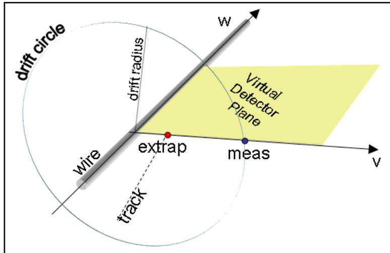
The Kalman weighted average is made between the PCA extrapolated point and the measured point, given by the intersection of the drift radius with the (v-w) plane
