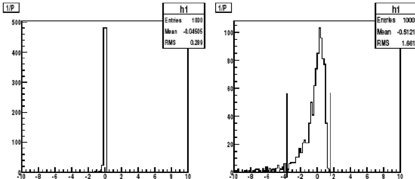
Figure 10: Pull distribution  $\Delta(1/p)/\sigma$  for 1 GeV muons after passing through the PANDA straw tube detector. Left: Standard GEANE result ( $\text{RMS} \simeq 0.3$  in the displayed window); right: result after the modification with  $\alpha = 0.995$  (see the text). The region between the vertical lines has  $\text{RMS} = 1.03$ .
