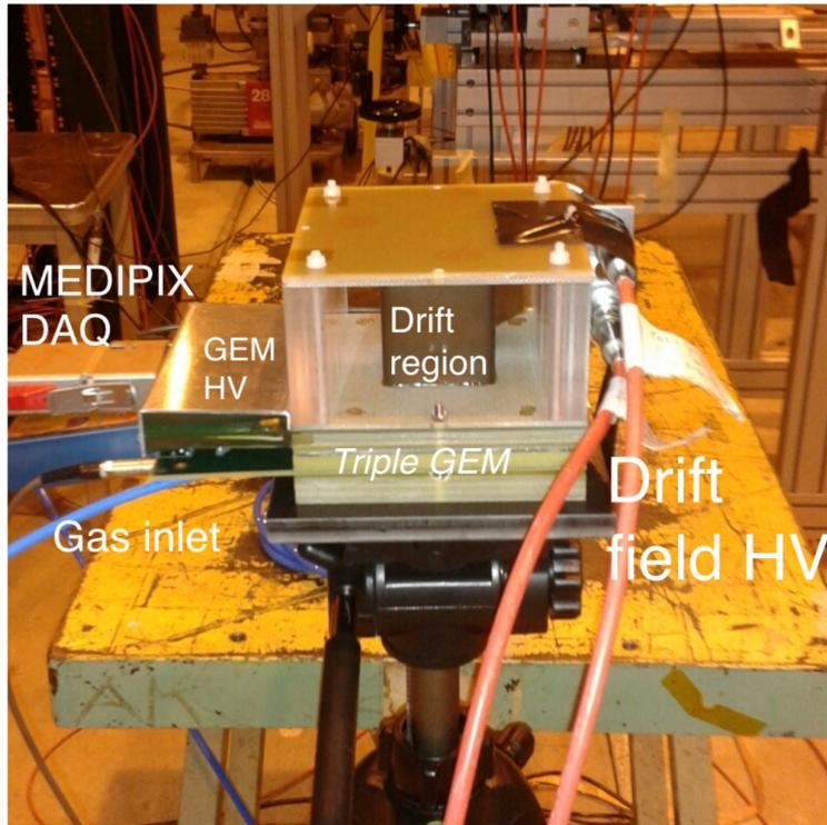
Anode is an ASIC used to read-out signals from **four** 512x512 **55 $\mu$ m** silicon pixel sensors (MEDIPIX)
