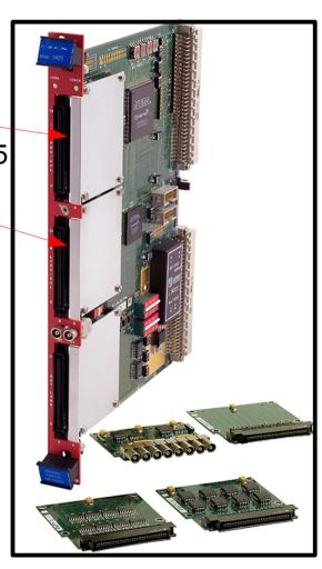
CAEN V1495: includes an FPGA that provides ASIC Configuration and DAQ 3
