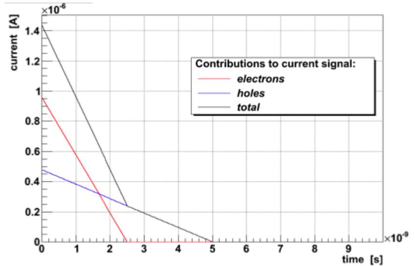
Pulse after front-end preamplifier
