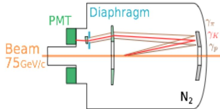
Cherenkov light is emitted with an angle of  $\vartheta = \arccos\left(\frac{1}{\beta n}\right)$  where  $\beta = v/c$  and  $n$  is the refraction index
