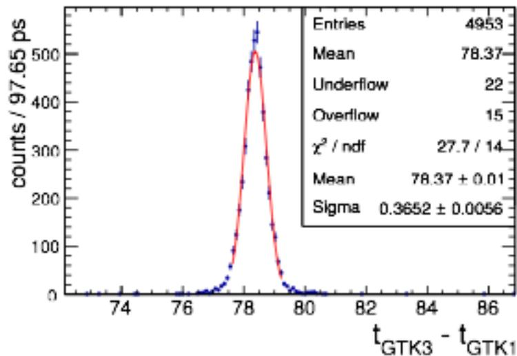
Time resolution by measuring the time difference between hits in two stations with a bias of 200 V:
