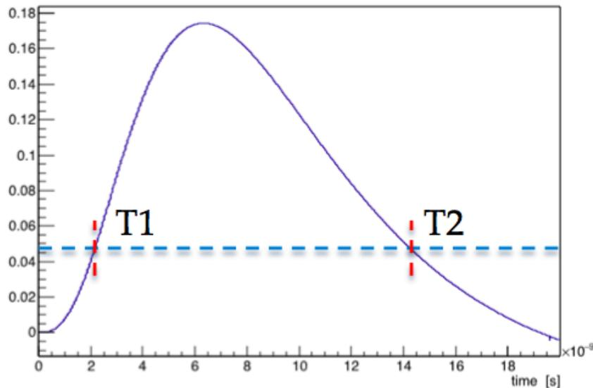
Typical signal at the amplifier output
