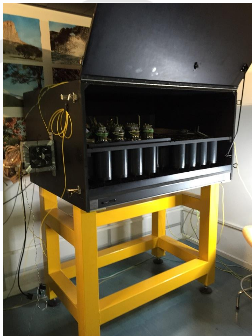
DarkBox for PMT tests
