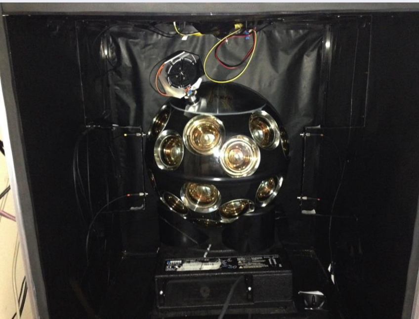
Green box for acceptance test and calibration of the DOM
