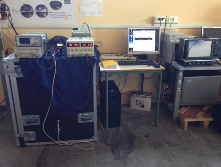
Green box for acceptance test and calibration of the DOM
