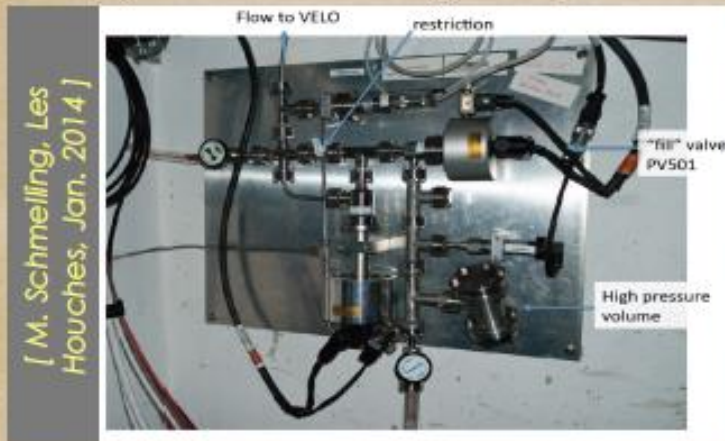
System for Measuring Overlap with Gas
