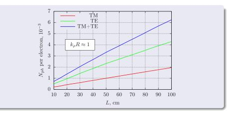
The radiation power grows with the increase of the crystal length L. For example, at  $k_{\rho}R \approx 1$ and L = 1 m for the same bunches it will be about 160 MW.
