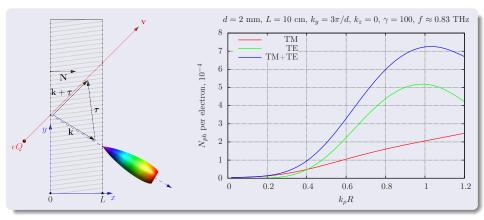
Intensity of radiation in diffraction direction reaches its maximum at  $k_{\rho}R \approx 1$ , which corresponds to wires radius of  $R \approx 65 \ \mu \text{m}$  if crystal period  $d = 2 \ \text{mm}$ . For an electron bunch with  $n_e \sim 1.25 \cdot 10^9$  and  $t_b \sim 30 \cdot 10^{-15}$  s (SwissFEL parameters) instantaneous radiation power in case  $k_{\rho}R \approx 1$  will be  $P \approx 18 \ \text{MW}$ .
