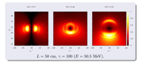
For large  $k_{\rho}R$  contributions of the TE- and TM-polarized waves to the total intensity of radiation can be comparable (in considered case  $k_{\rho}R \sim 1$  contribution of TE-wave is dominant), whereas for thin wires  $(k_{\rho}R \ll 1)$  only TM-polarized wave contribute noticeably to the total radiation intensity.
