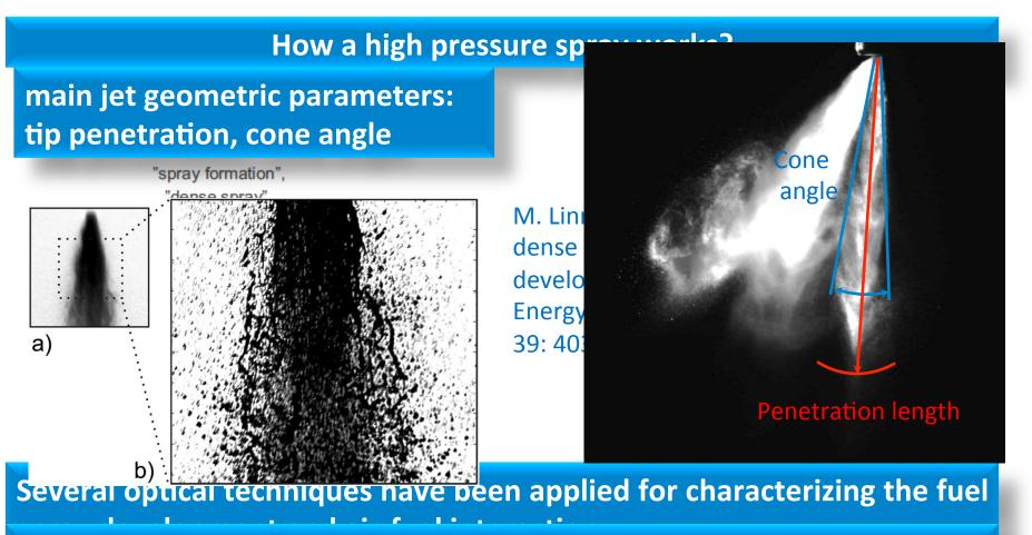
measurements about the internal structure of the spray results quite complicated, especially in the dense region close the nozzle
