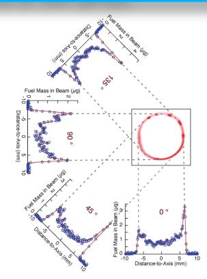
X-radiography of hollow-cone direct injection fuel spray
