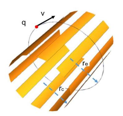
Grating consists metallic strips with width *a* and with the separation *b*
