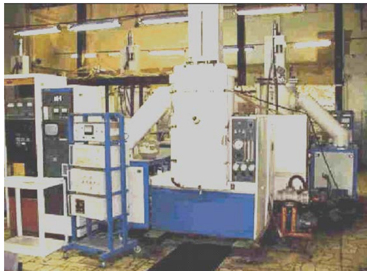
Crystal growth puller Crystal-3M, 1,165 deg C melt
