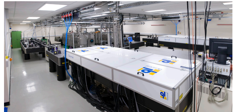
Gemini 2 beams TiSa System 15J in 30fs, 20s Rep. Rate
