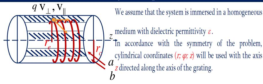
We consider the radiation of a relativistic charged particle q, moving along a circular helical trajectory of radius  $r_e$  inside a infinitely long coaxial cylindrical grating. The latter consists metallic strips with width a situated on the rings with radius  $r_c < r_e$ . The distance between the strips will be denoted by b.
