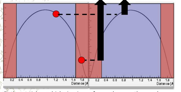
Both particles which impinge far and near the nuclear corridor interact with nuclei and suffer nuclear dechanneling.
