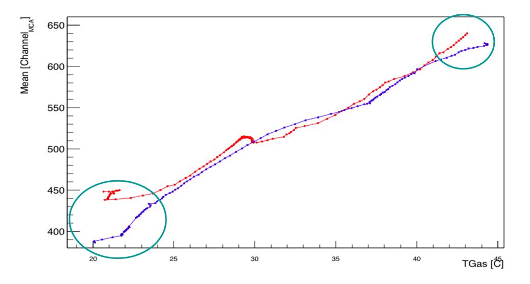
!!! For the DROP and RISE phase the gain increases in a quite linear way
