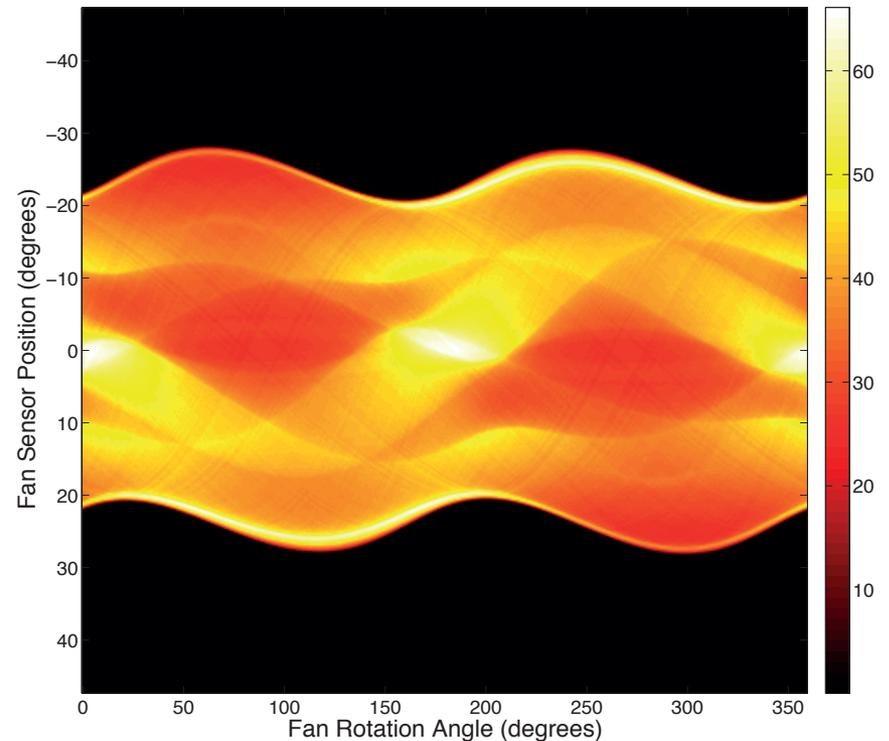
Reconstruction: Inversion of Radon transform:
