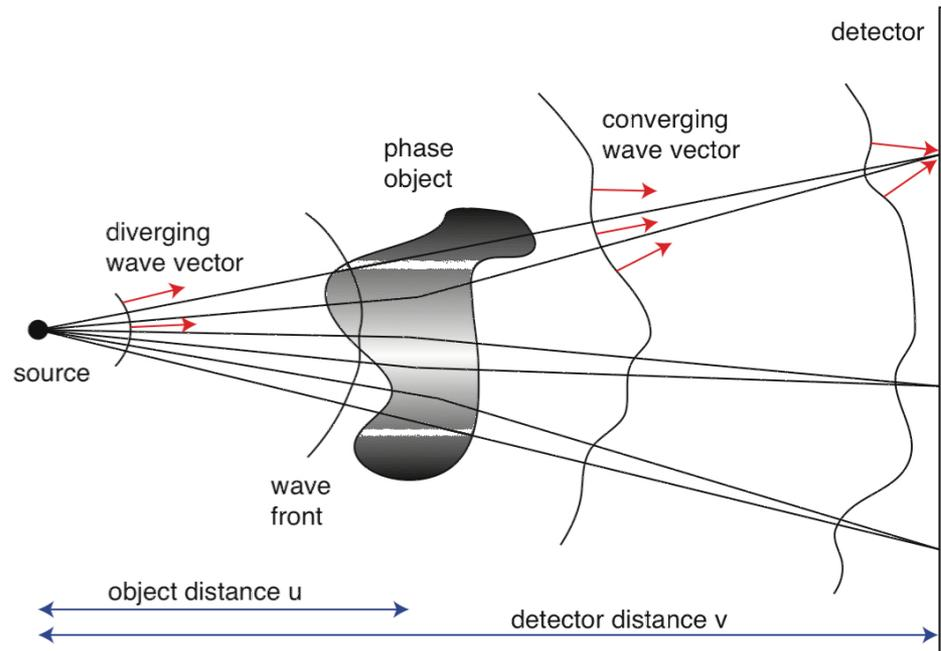
The intensity distribution on the detector is a result of wavefront distortions introduced by phase object. The Transport of Intensity Equation relates sample thickness to measured intensity distribution:
