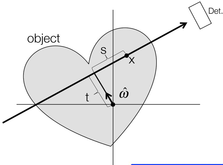
Parametrize each point on ray by a normal unit vector  $w$ , distance to rotation center  $t$  and longitudinal position  $s$ :
