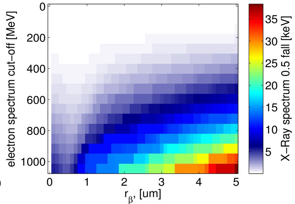
Overall betatron spectrum depends on energy and injection radius distribution of the electron bunch  $\Rightarrow$  numerical calculation necessary.
