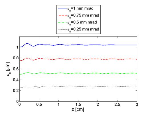
The matching condition we used gave a good result in a simulation scan at various emittances
