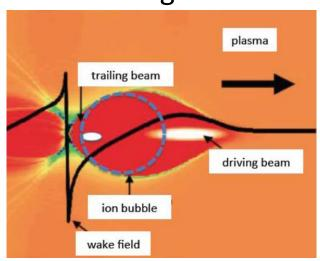
In the bubble regime it is not possible to minimize the energy spread, because of the spike localized at the end of the bubble
