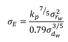
The minimum energy spread occurs by injecting a very short bunch ( $k_p\sigma_z\approx 0$ ) injected on crest ( $\varphi=0$ ) with a minimal spot size ( $k_p\sigma_r\approx 0$ )
